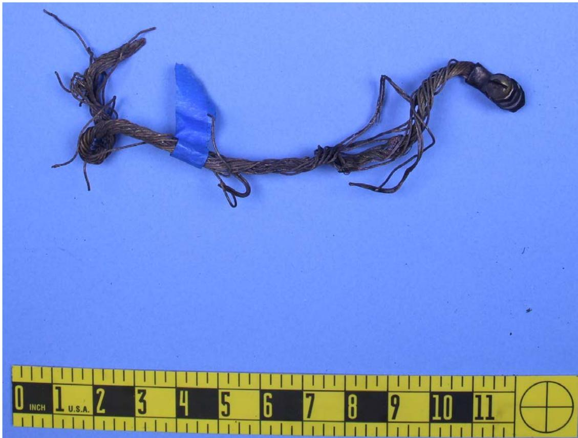
Figure 7. Overall photograph of STC fuse to bus bar.
