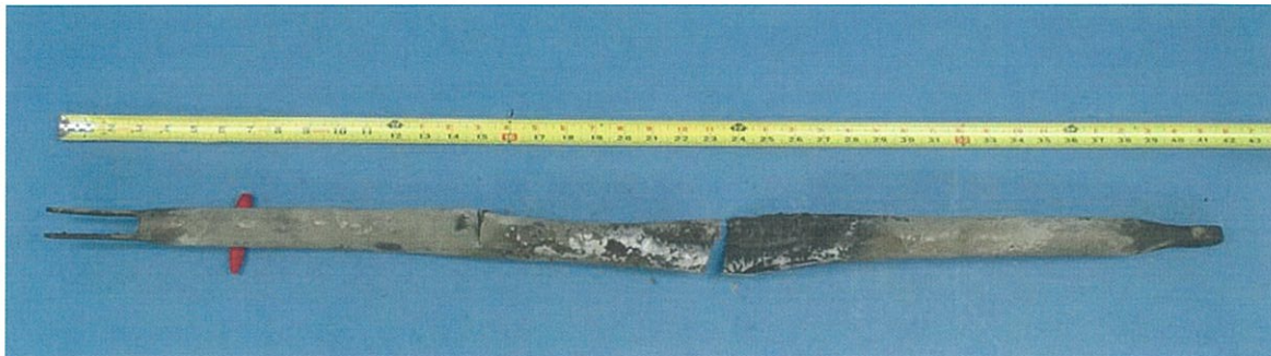
Figure 2: Left aileron control rod
