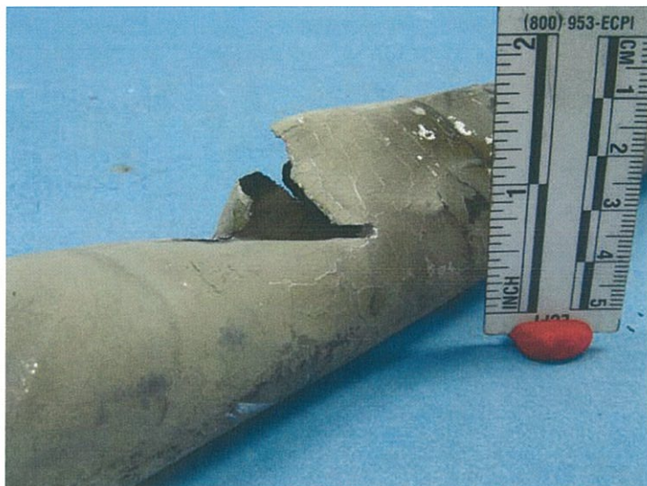
Figure 4: Tear on the portion of the aileron control rod with the yoke
