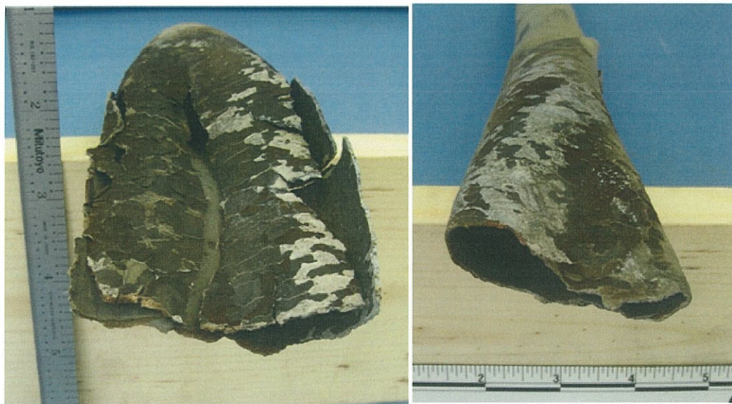
Figure 3: Severed ends of the aileron control rod
