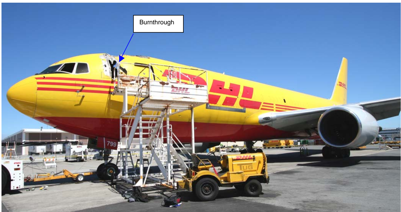
Figure 1: Exterior view of the accident aircraft showing burn-through damage at lavatory location.
