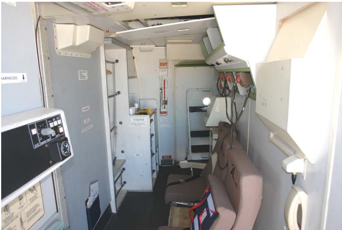
Figure 18: Supernumerary compartment of an exemplar aircraft. Panels removed on from of bulkhead containing oxygen mask stowage boxes.
