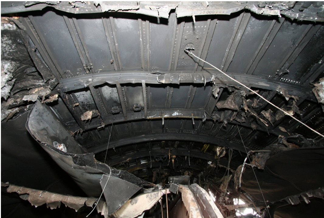
Figure 9: Ceiling cargo liner missing above cargo positions 1 and 2
