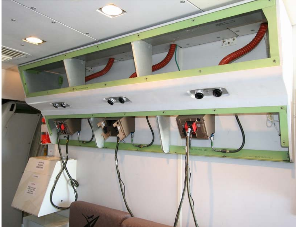
Figure 25: Exemplar bulkhead containing oxygen mask stowage boxes, lights and vents. Face panels of bulkhead have been removed in photograph.
