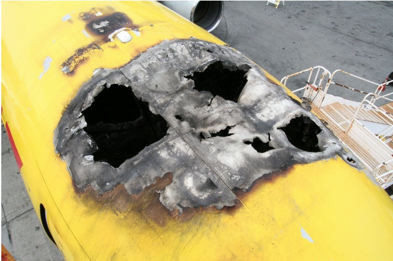
Figure 2: Burn-through on crown of accident aircraft centered over the supernumerary compartment
