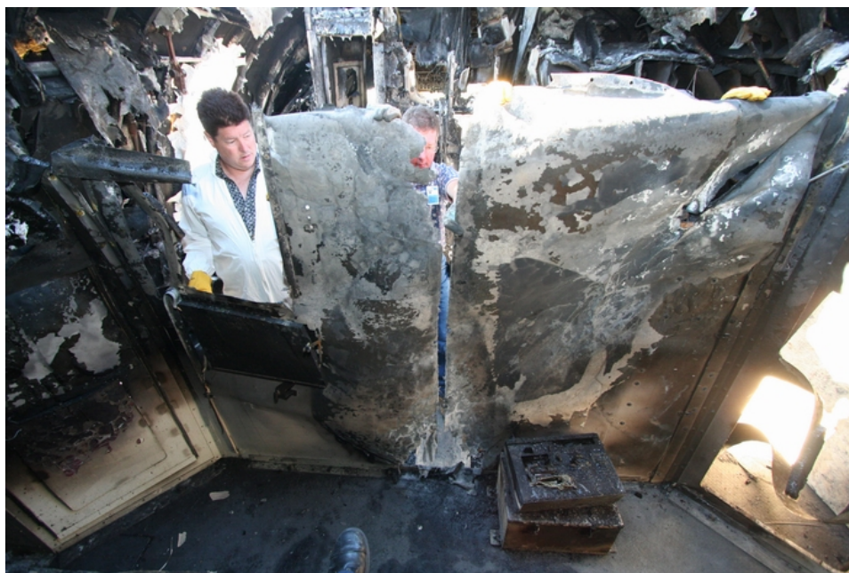
Figure 11: Aft facing side of smoke barrier wall. The wall is being held up in place after the loose fire debris had been removed from the area.
