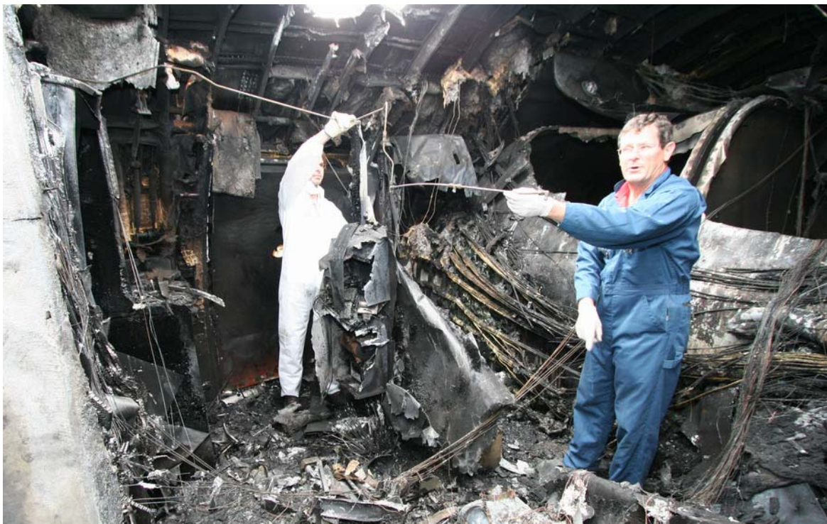
Figure 27: Stainless steel oxygen supply line in supernumerary compartment, held in position by investigators
