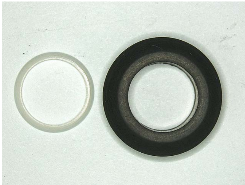
Figure 2: New elastomeric packing (black) and nylon packing retainer (white)
