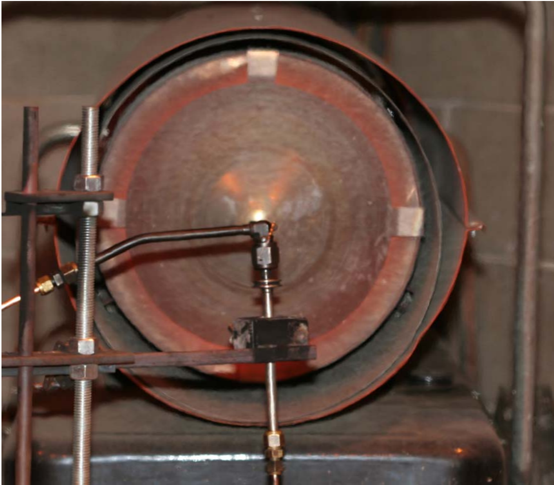
Figure 14: Forced air combustion heater test setup
