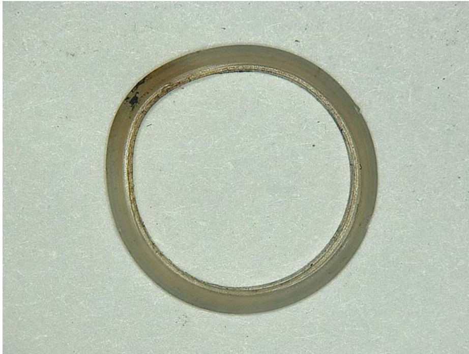
Figure 13: Nylon packing retainer after the second oil burner test
