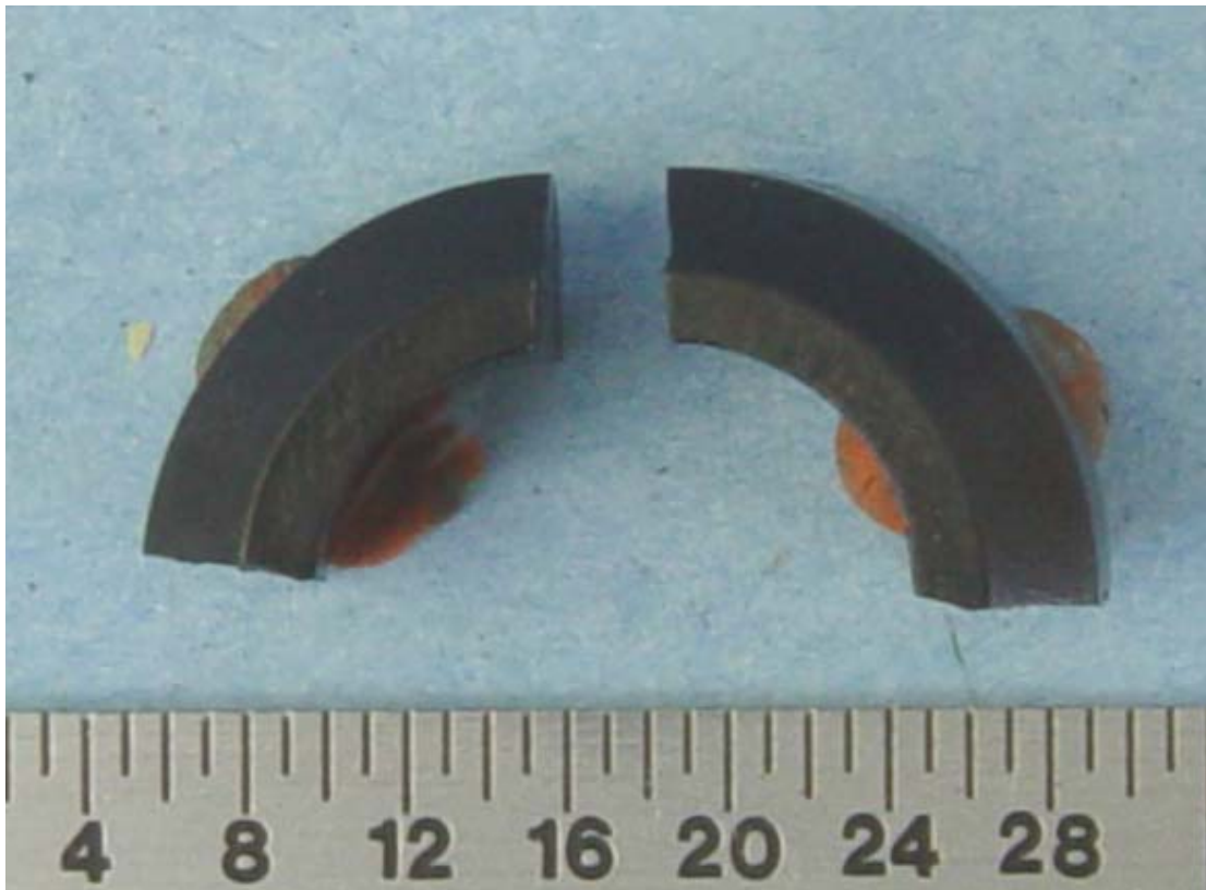
Figure 4: Fractured elastomeric packing after squeezing. The packing had been exposed for a total of 9 minutes to the 600 degree F environment.
