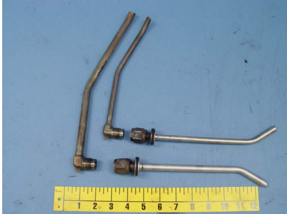
Figure 1: Primary (3/8" OD) and secondary (1/2" OD) fuel manifold fittings from the left hand side of the engine
