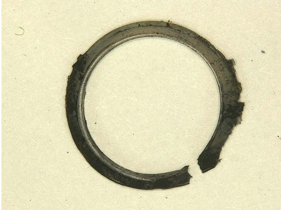
Figure 10: Nylon packing retainer after the first oil burner test
