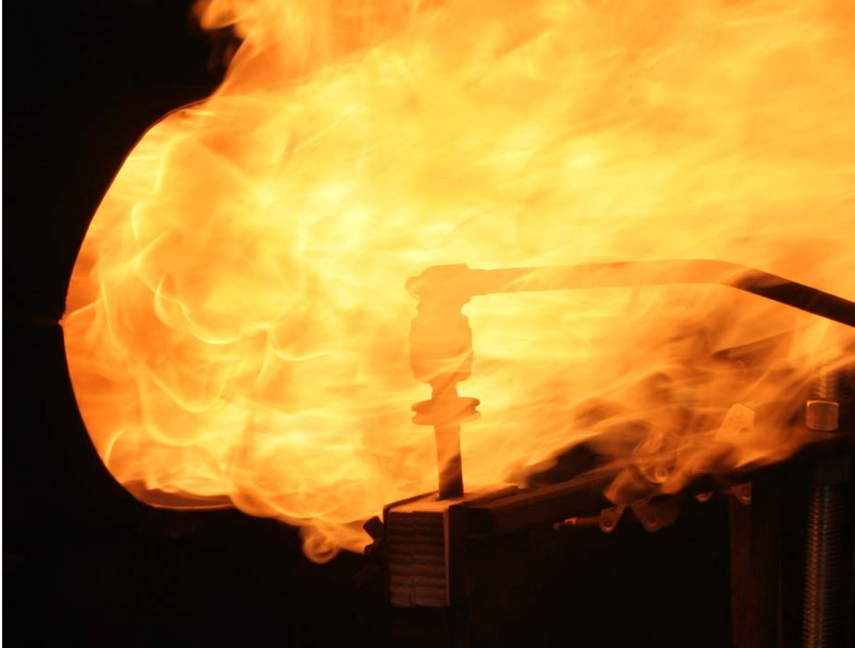
Figure 7: Fuel fitting exposed in oil burner flame
