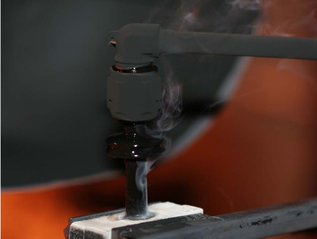
Figure 8: Fuel fitting leaking under 300 psi static pressure at the end of the test.
