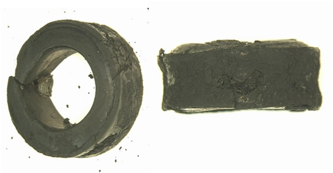
Figure 9: Two views of the packing removed from the fuel fitting after the first oil burner test
