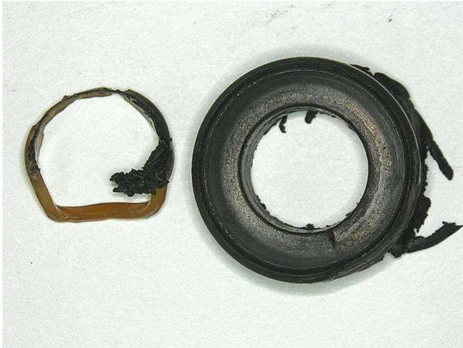
Figure 17: Packing and packing retainer after disassembly of the fitting at the conclusion of the second combustion heater test
