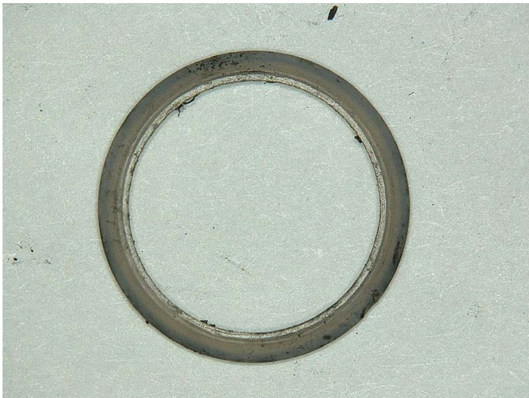
Figure 16: Nylon packing retainer after the first combustion heater test
