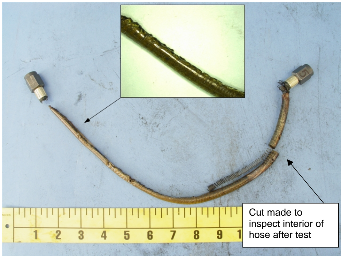
Figure 10: Hose assembly after Test #5 (over braid removed for clarity)
