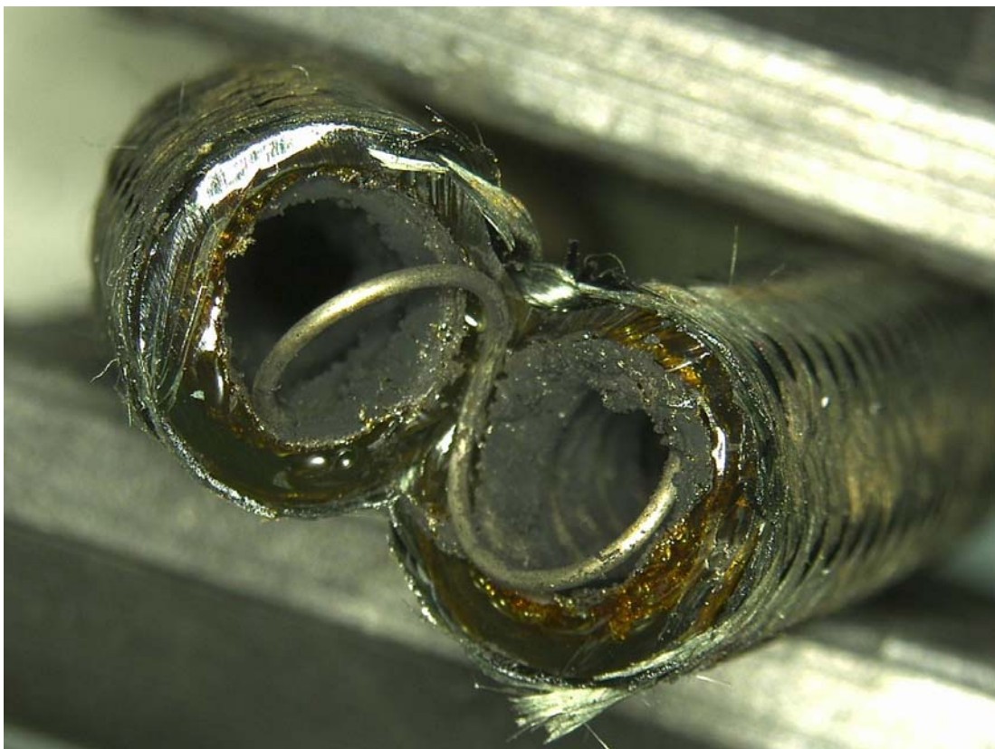
Figure 7: Soot coating the inner surface of the hose from Test #3
