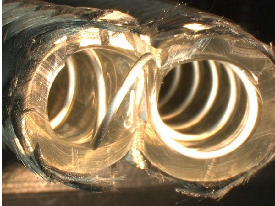
Figure 3: Interior of flexible hose after Test #1
