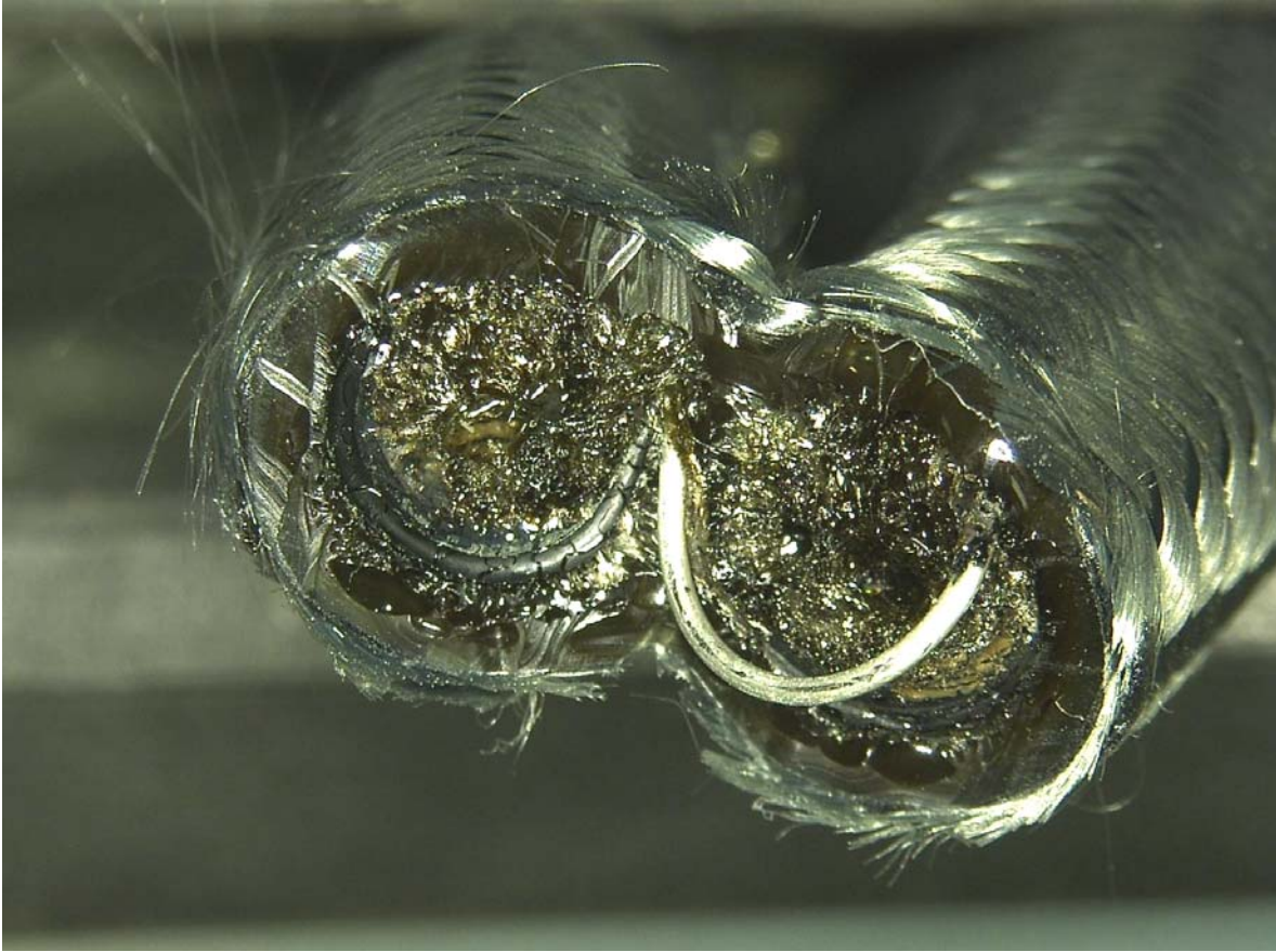
Figure 5: Sponge like material on inside of flexible hose after Test #2
