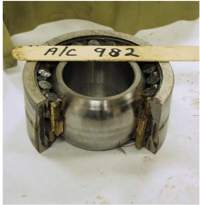
Figure 26--Left corrosion visible on the inner spherical race of the pivot bearing after cleaning. A similarly opened bearing from another jackscrew assembly is shown at right for comparison.
