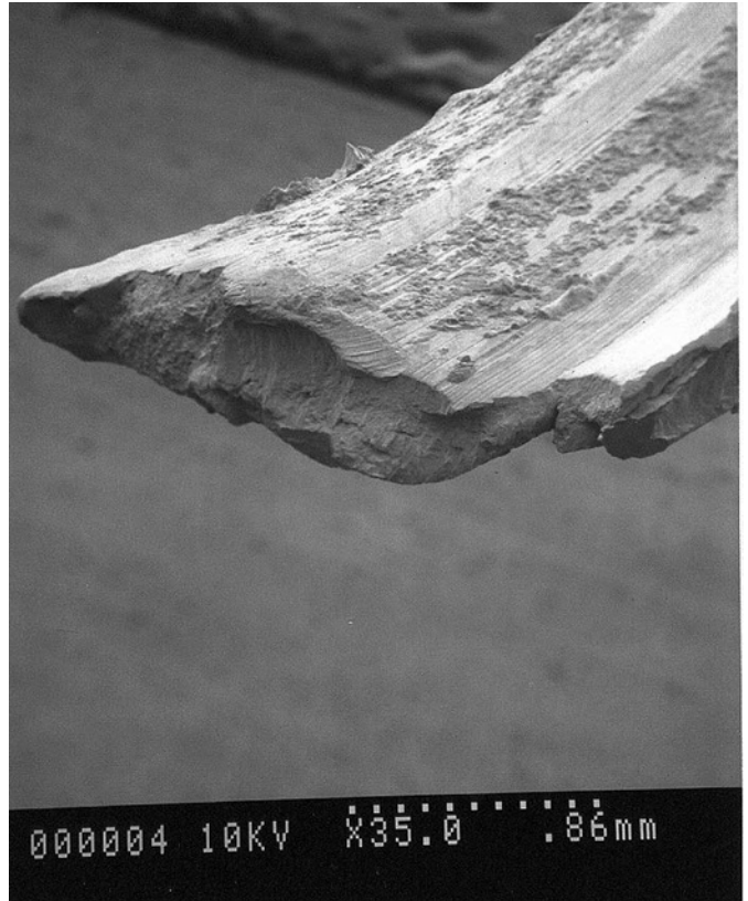
CLOSE-UP OF TRANSVERSE FRACTURE. (NEG: 00-S0072)
