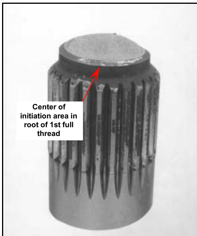
Figure 69--Closer view of the torque tube fracture initiation area showing the reflective band (between arrows) adjacent to the thread root.
