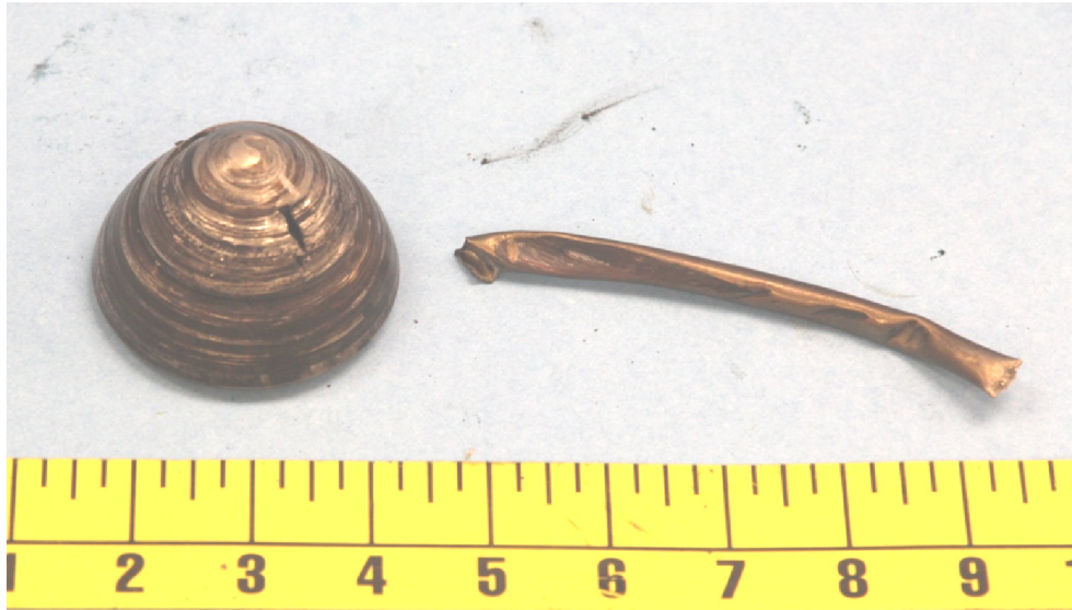
Figure 1. The nose cone at left showing rotational marking and the crushed and abraded tube at right.
