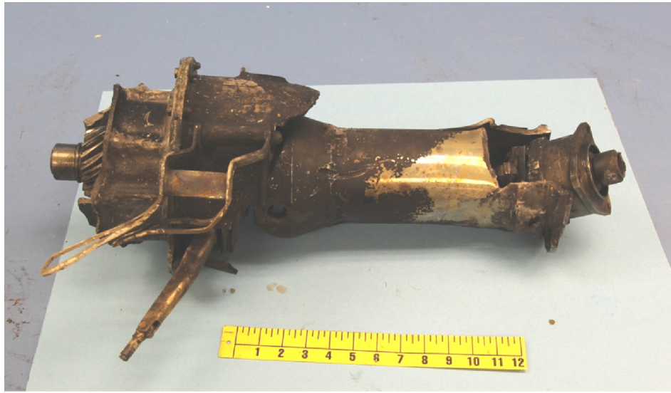
Figure 5. The fractured transmission input shaft inside the linking tube
