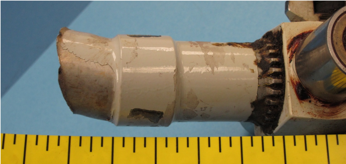
Figure 1. Upper view displays the as-received components. Middle view shows the bending deformation in the mast above the fracture. View at left shows the fracture face.
