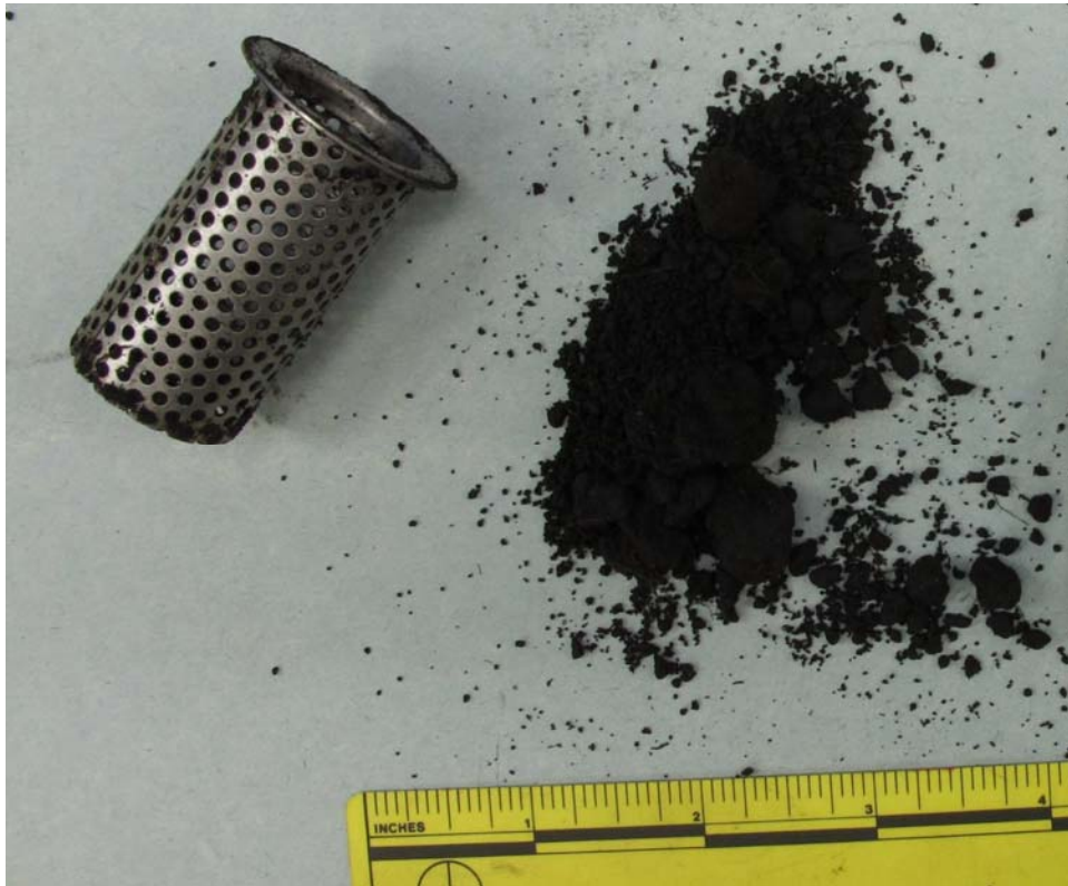
Figure 1. Overall picture of tail rotor gearbox filter and debris.
