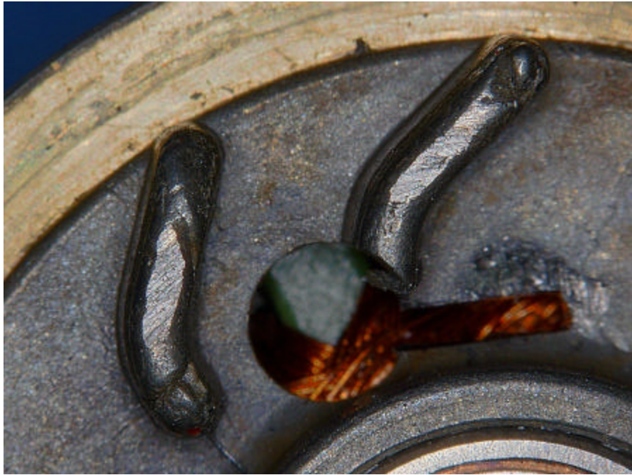
Figure 5. Smearing on fins of gyro
