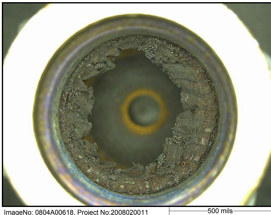
Figure 2--A view inside the filter housing at the remaining filter cloth material.
