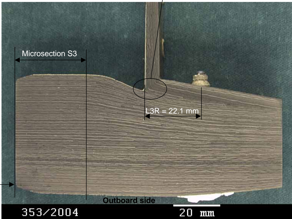
Fig. 7: Delamination starting from crack at rib #1, further delamination starting at bush-hole (arrow), loc. of microsection S3, delamination length L3R, section S3-S3
