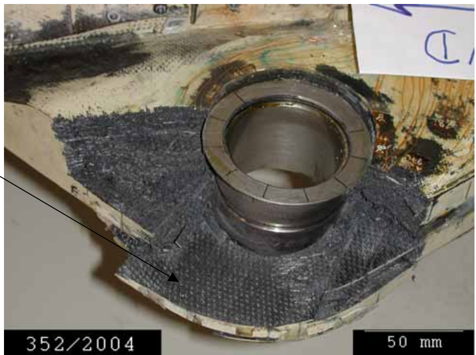
Fig 3: Lug Test # 3, fracture path, view from inboard side, condition: after test and partly separation of fractured parts
