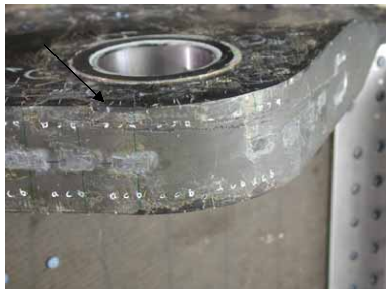
09368/03 09369/03 Fig. 5: Delamination path, trans laminar fracture path (arrow), view from lower side, condition: after static test
