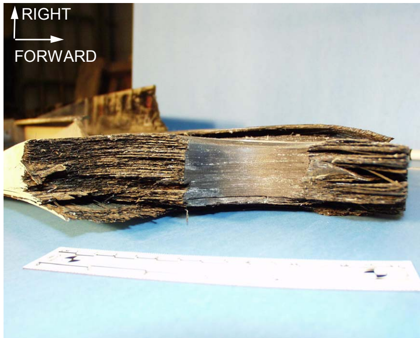
Figure 46. Upper fracture surface of the left forward lug, viewed looking up.
