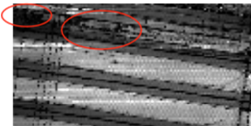
Figure 1.16 Ultrasonic attenuation image of left side tail region K.
