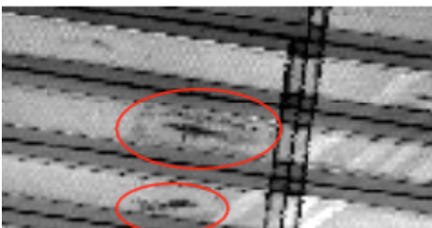
Figure 1.11 Ultrasonic attenuation image of left side tail region F.
