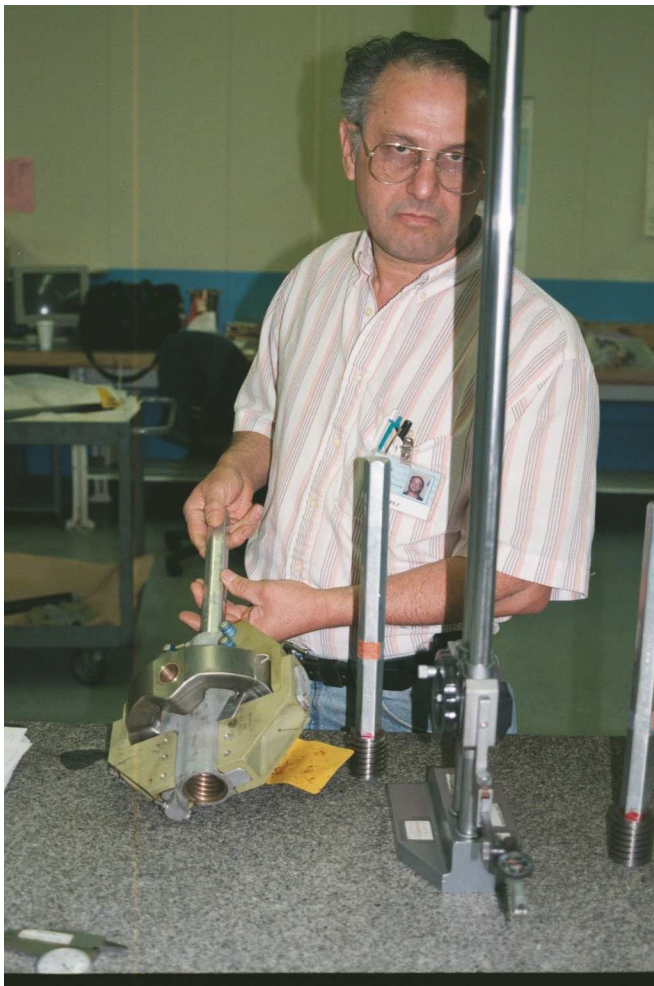
Figure 7. Performing a functional check on the nut with Go No-Go gaging.
