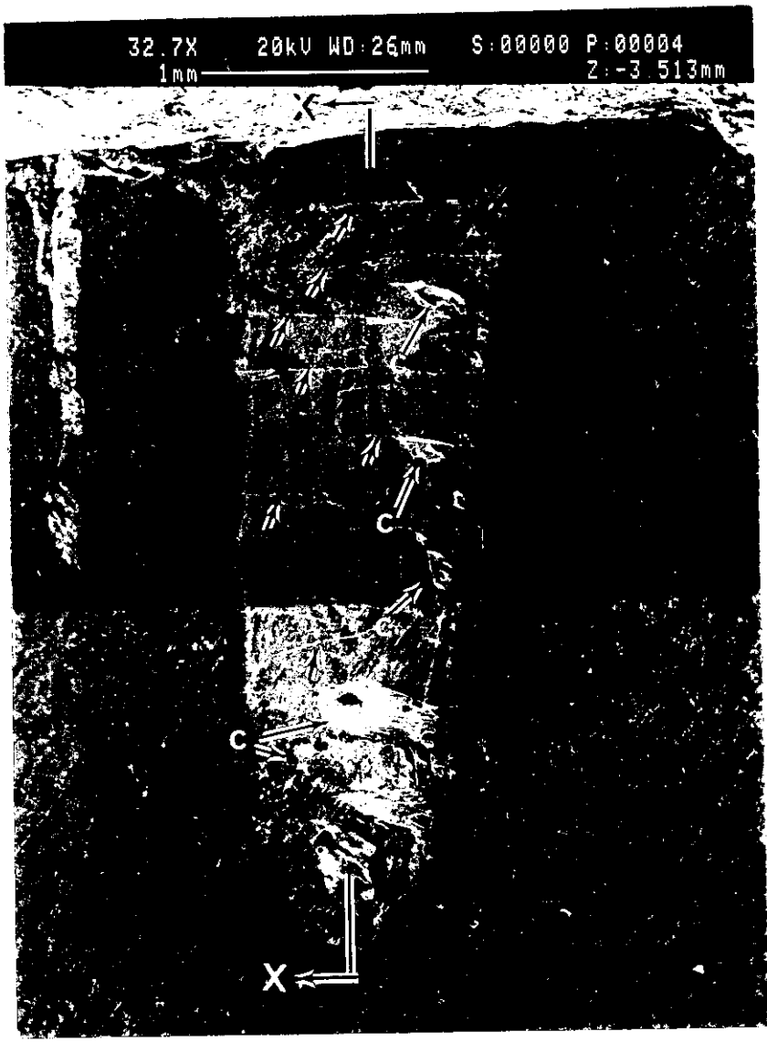
Figure 11. Composite photograph showing an SEM view of scuff marks at and near the fracture origin area "o2". Note numerous parallel cracks (ladder cracks) within the main scuffed area, some of which are shown by the arrowheads.
