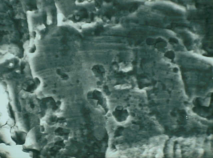
Materials Laboratory 15 - Exhibit No. 15A - Photo 5. SEM photograph of a fracture area containing a fatigue striation pattern.
