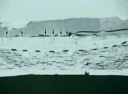
Materials Laboratory 15 - Exhibit No. 15A Photo 2. Fatigue crack region on the cut-out piece. The bracket indicated mechanical damage, and the arrowheads indicate origin areas, and the extent of preexisting cracking is indicated by the dashed line. (3X)
