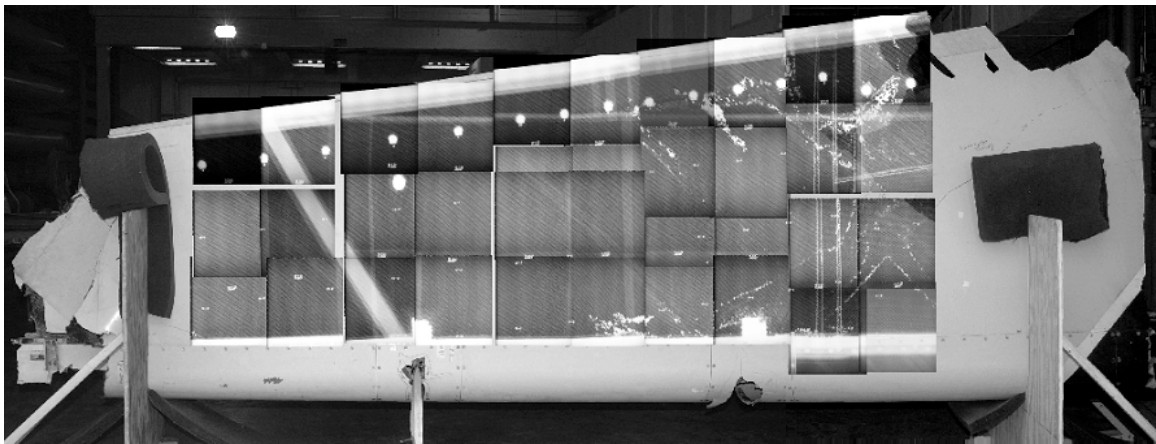
Figure 3.02 Compilation of radiography results superimposed on picture of the section of rudder examined.
