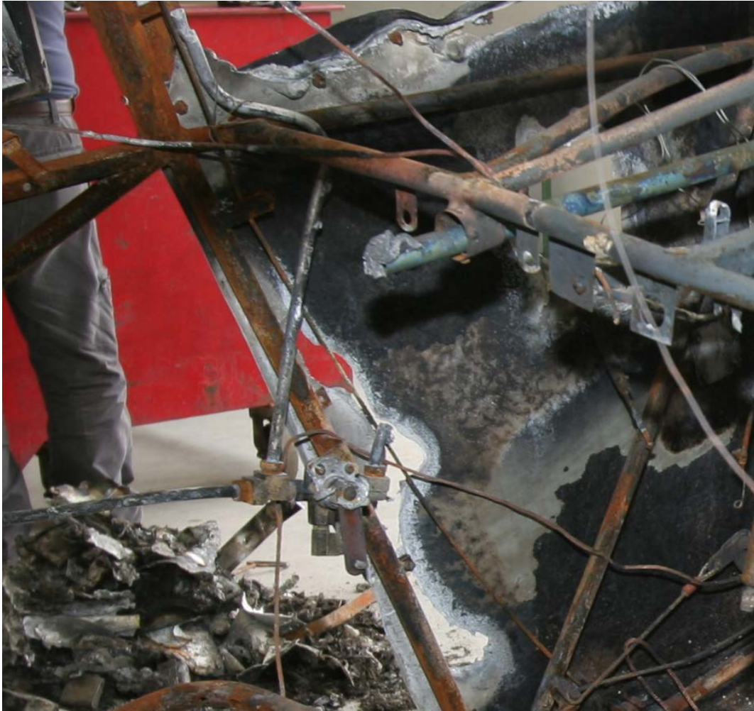
Figure 3: Fuel selector valve with input from right wing tank missing and output fuel line also missing.
