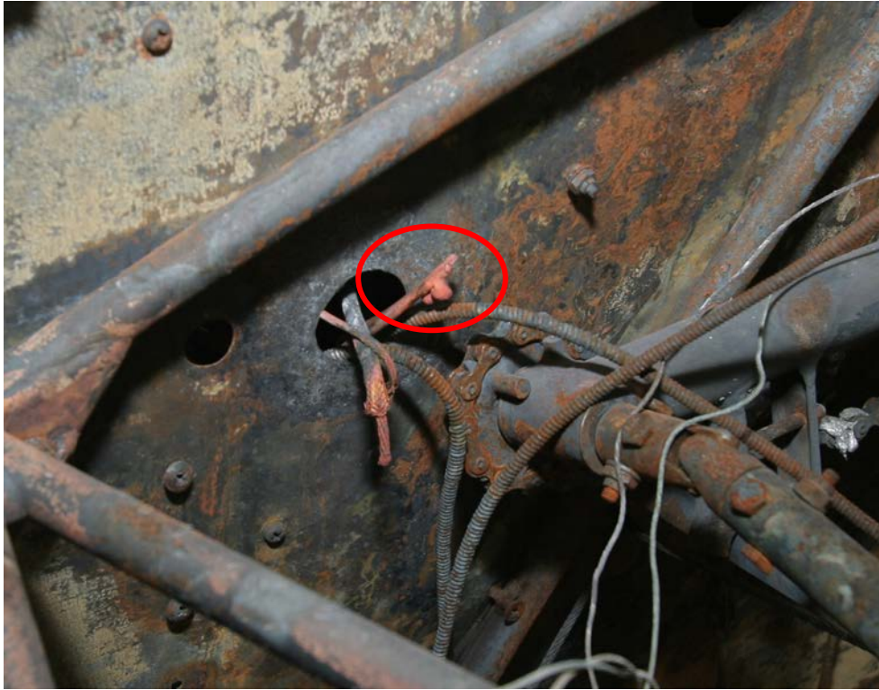
Figure 4: Melted engine primer pump fuel lines protruding into the cockpit from the engine compartment firewall.
