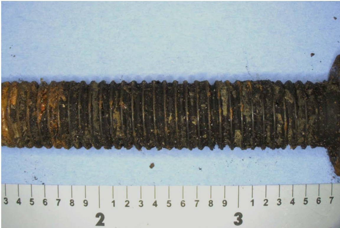
Figure 2. Fuel pump housing bolt found unattached from housing.
