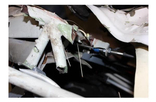
4- Throttle cable fractured bracket on the airplane
