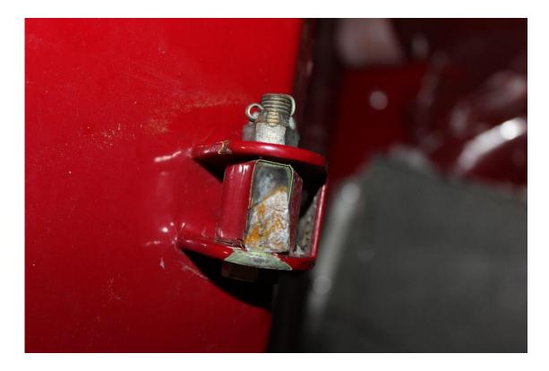
2- Left wing strut fracture, attached to airframe mount
