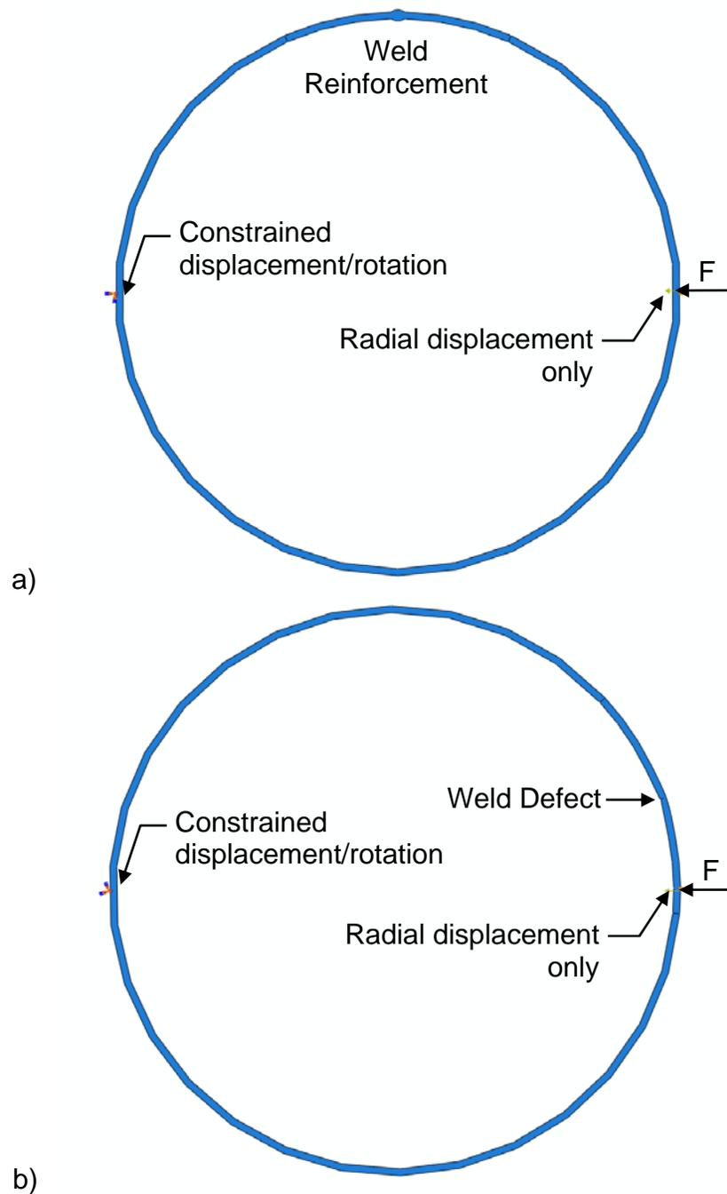
Figure 3: Finite element models and boundary conditions used in determining the effects on the pipe from loading by the winch on the sidewall of the receiving pit; a) a model similar to DSAW pipe with the weld reinforcement at the top; b) a model similar to the geometry of pup 1 with the weld defect  $71^\circ$  from the top of the pipe.
