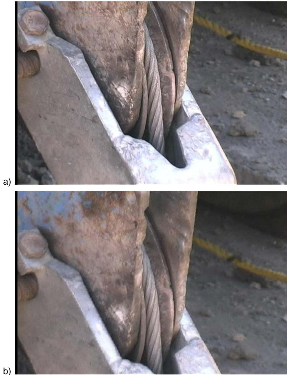
Figure 4: Video frames showing motion of the cable as it pulled the bursting head toward the receiving pit. The frames were separated by 1.12 s. The images were calibrated using the diameter of the cable (0.562 inch).
