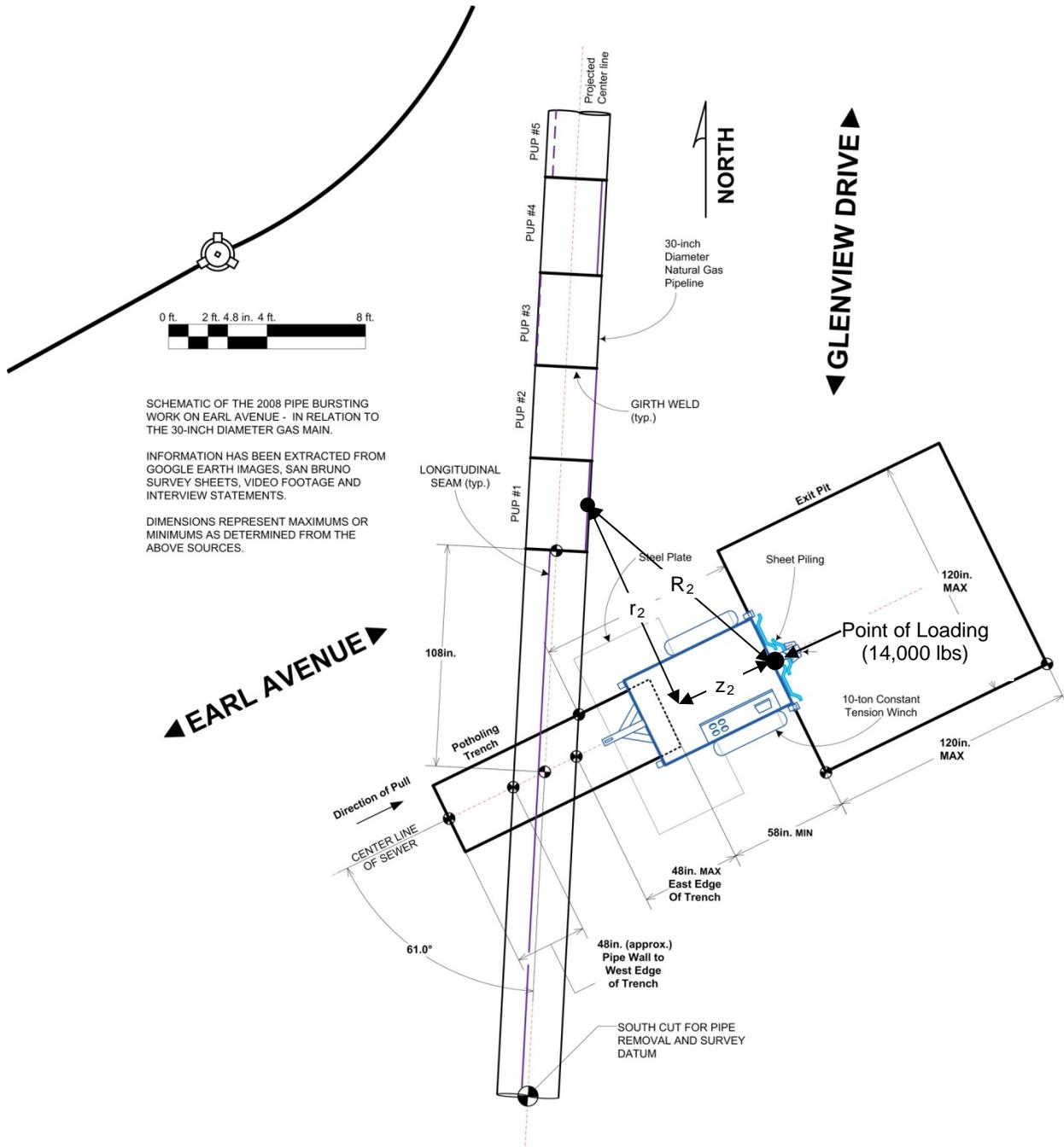
Figure 2: Same as figure 1 showing the distance between the winch brace and the initiation point on pup 1. The lengths  $r_2$  and  $R_2$  are projected onto the road surface.
