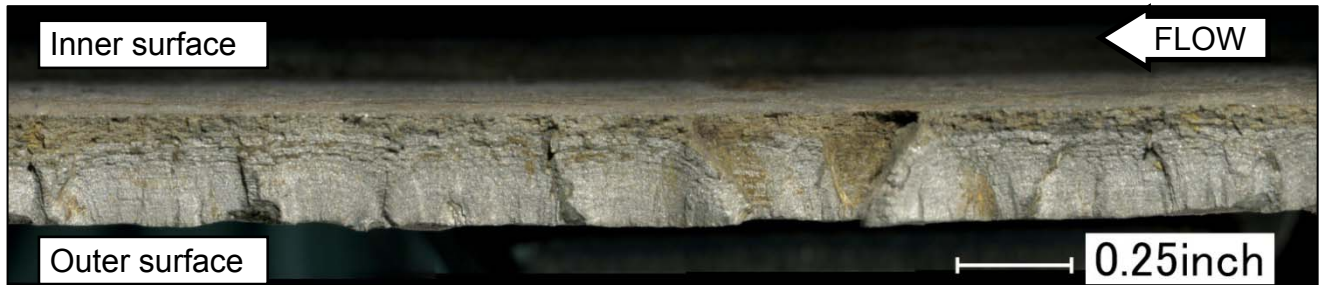
Figure 20. Close view of the fracture surface at the area of deepest crack penetration after cleaning with oxide-removing chemicals.
