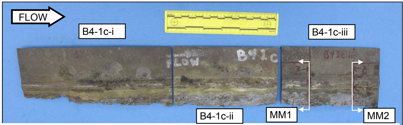
Figure 19. Overall view of the outer surfaces of pieces B4-1c-i, B4-1c-ii, and B4-1c-iii after cutting and cleaning with oxide-removing chemicals. Locations where metallurgical samples MM1 and MM2 were taken are marked on piece B4-1c-iii.
