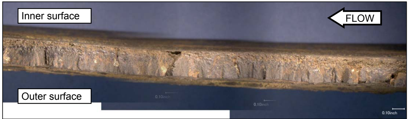
Figure 18. Close view of the fracture surface after cleaning with solvents and Alconox/water solution. Image is stitched together from 3 individual images using Stream Enterprise software by Olympus, Center Valley, Pennsylvania.
