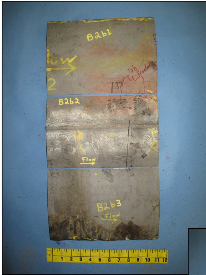
Figure 31. View of piece B2b2 cut from piece B2 to conduct lab fractures of crack indications detected by NDI.
