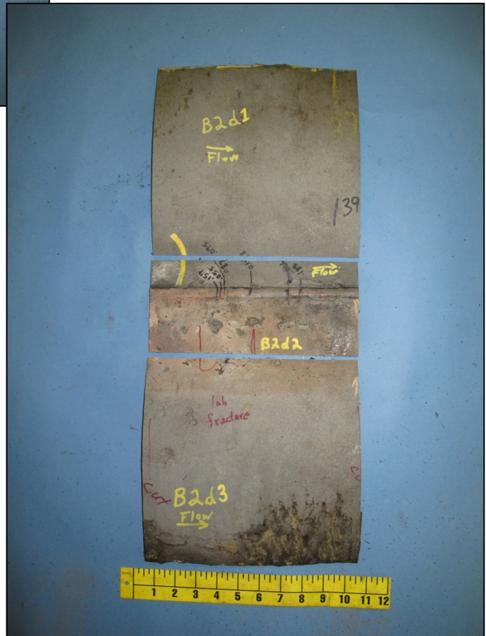
Figure 32. View of piece B2d2 cut from piece B2 to conduct lab fractures of crack indications detected by NDI.
