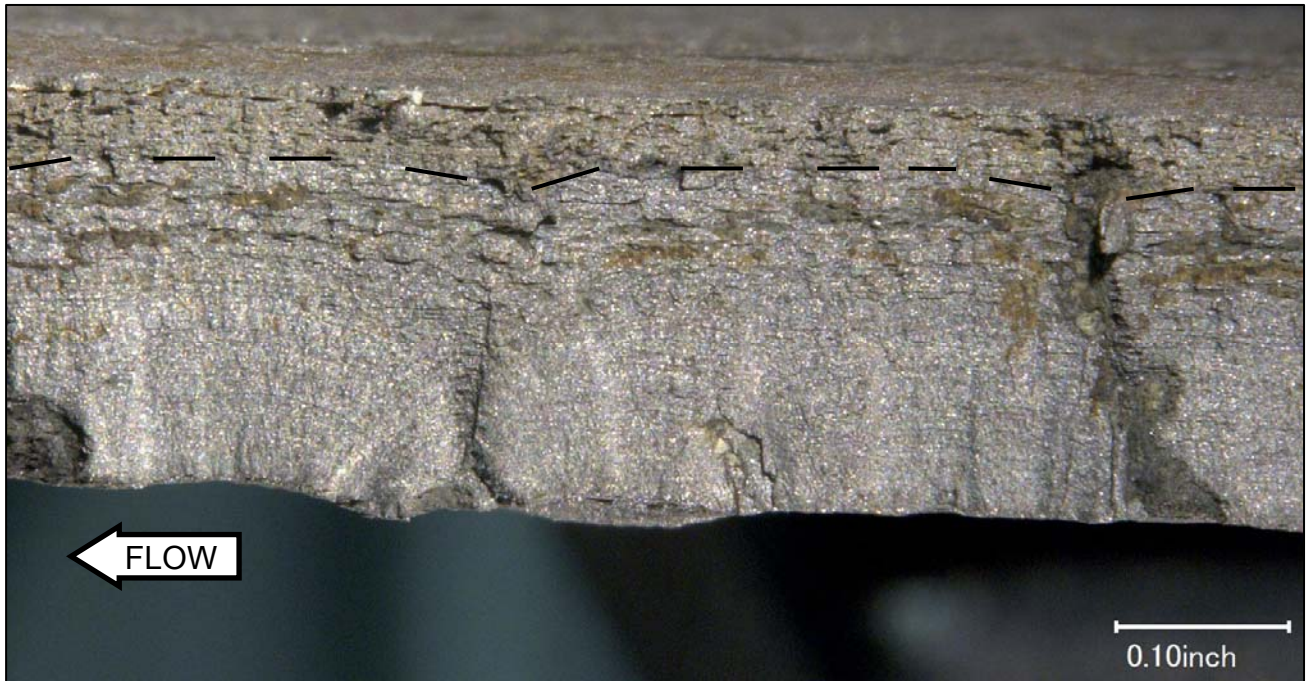
Figure 22. Close view of the fracture surface in the area of deepest crack penetration. A dashed line indicates the extent of the preexisting crack penetration.
