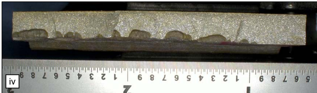
Figure 35. Overall views of lab fracture surfaces of samples B2b2ii-iv. The ruler is adjacent to the outer surface in each photo, and the pipe flow direction is from left to right.
