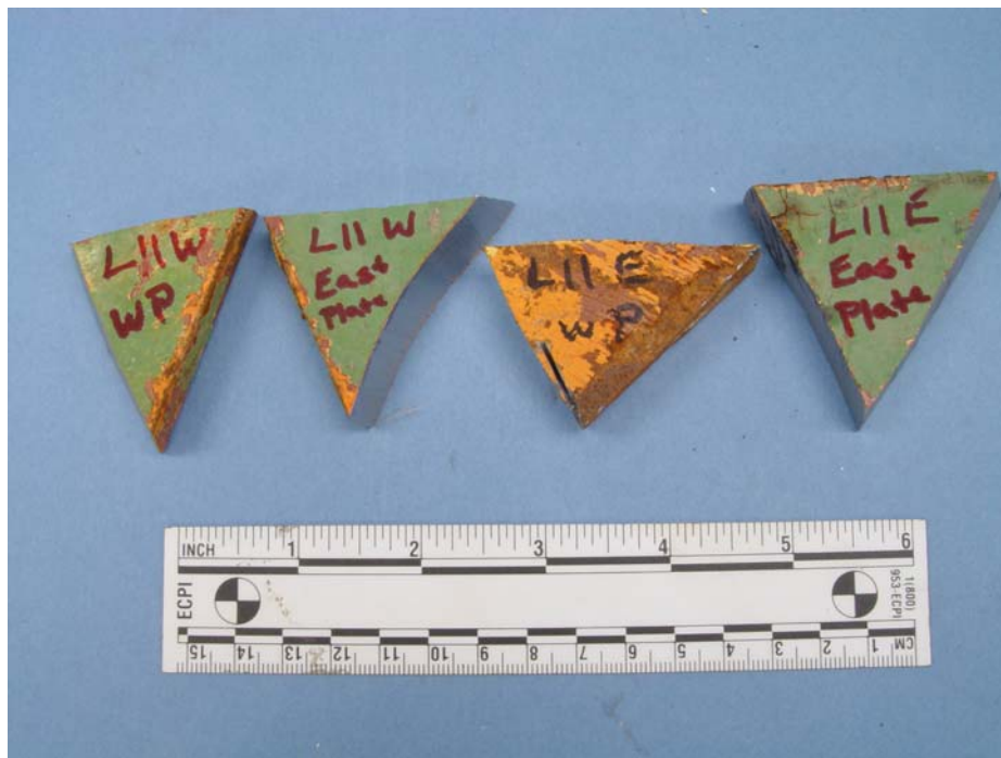
Figure 2: Portions cut from the L11 gusset plate.
