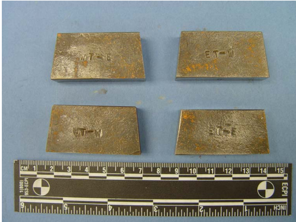
Figure 1: Portions cut from the U10 gusset plate.
