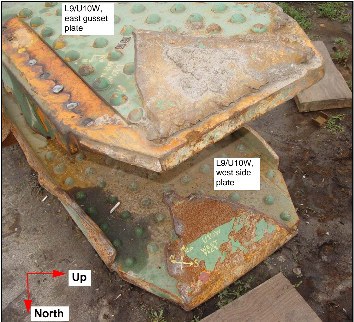
Figure 13. Photograph of the upper (U10W) end of diagonal L9/U10W showing the V-shaped tips of the gusset plates folded to the east. Photograph taken after removal of a piece of the east gusset plate for laboratory examination. The north, south, and up directions marked on the west gusset plate are oriented for the folded piece of the plate.
