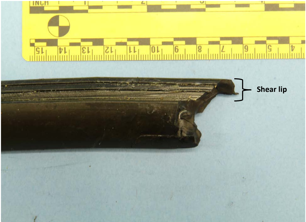
Figure 7. Close-up photograph of shear lip pattern.
