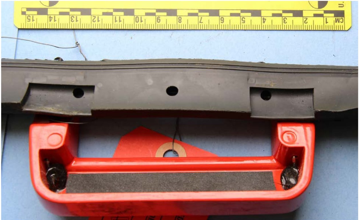
Figure 5. Photograph of molded cutouts in handle area of zip strip.
