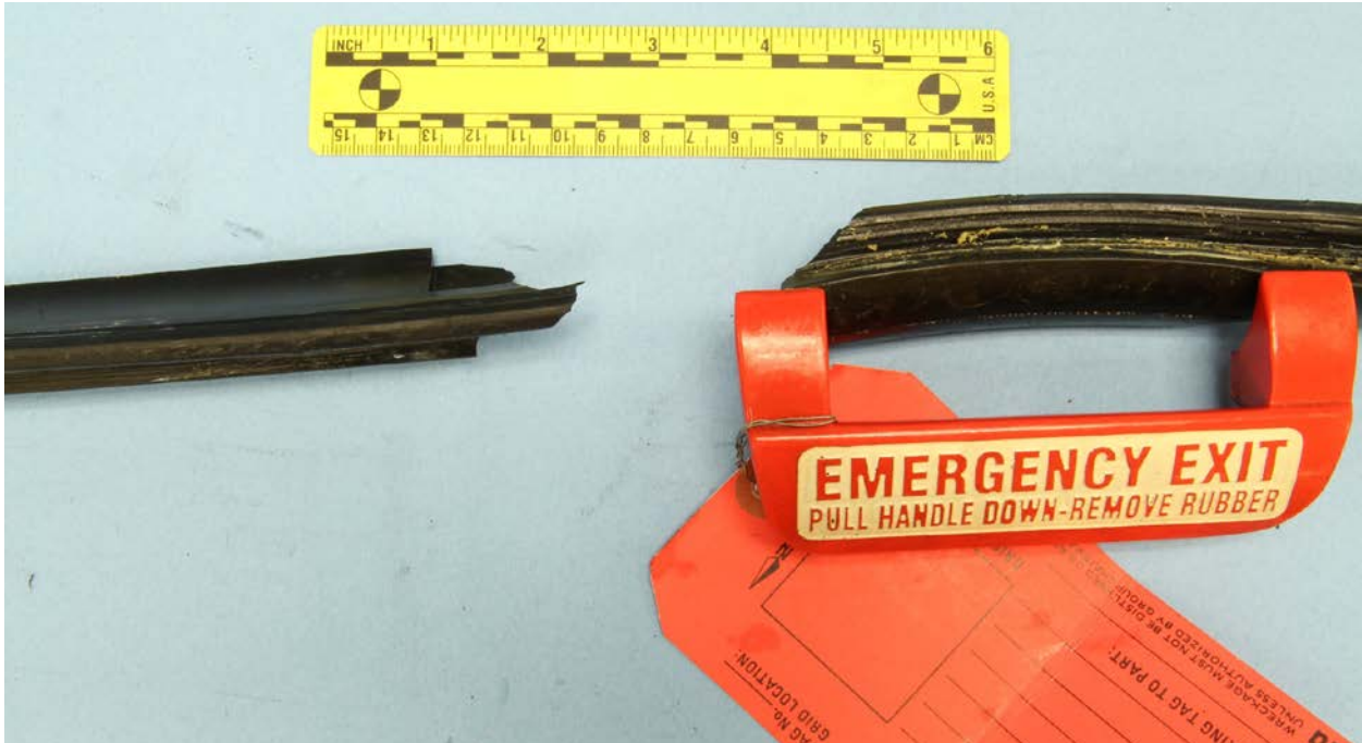
Figure 3. Photograph of full thickness (separation) tear (#4174 L9).
