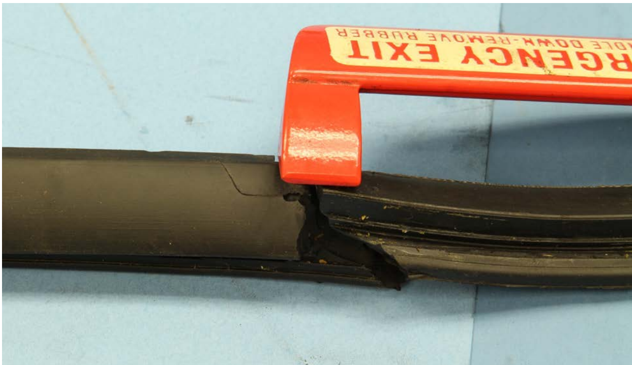
Figure 4. Photograph of partial thickness tear (#4196 R1).
