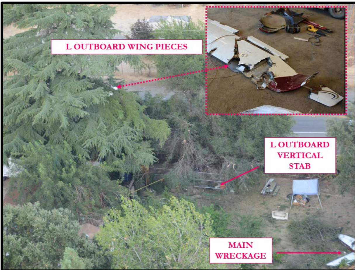
Figure 14: Debris Field Highlighting Left Wing Pieces
