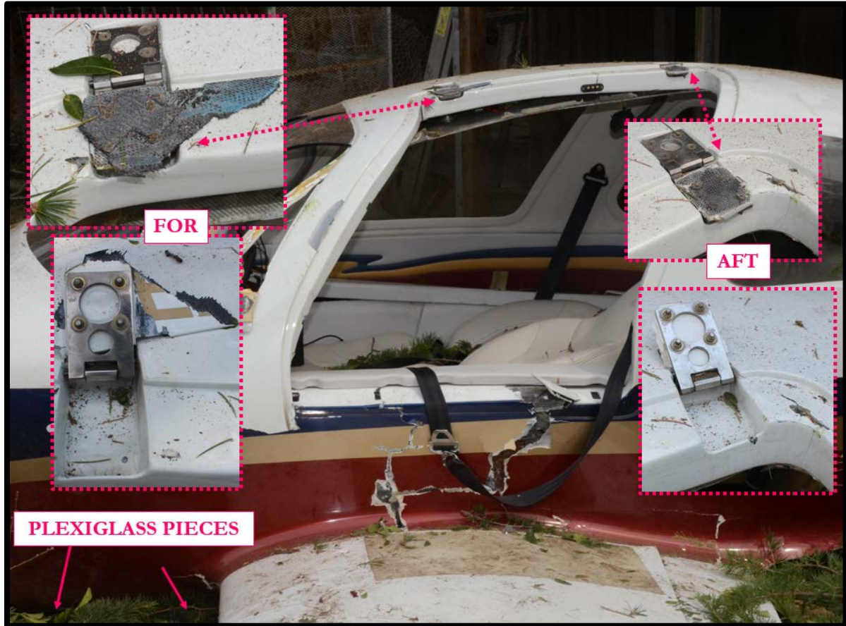
Figure 19: Accident Airplane Door Hinges
