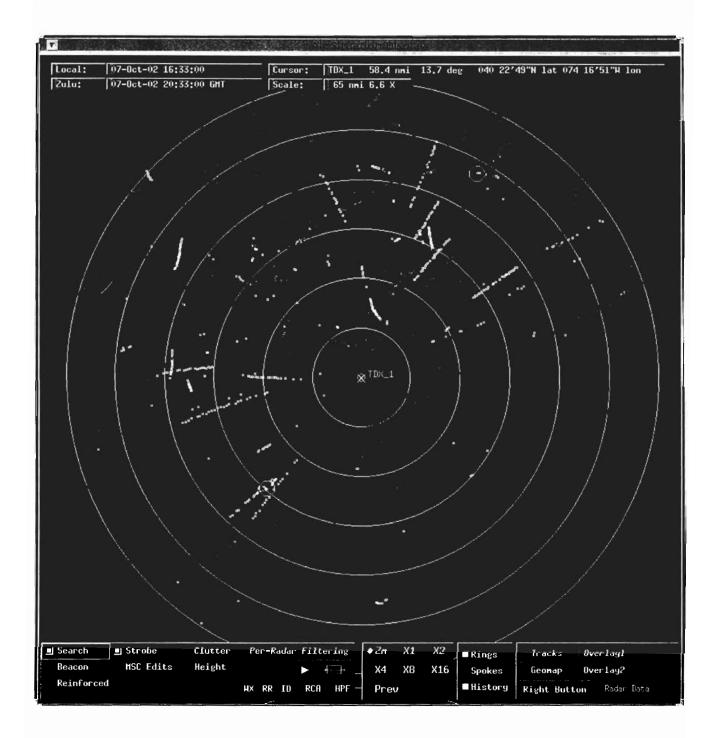
(2) Detected "raw" video replies can be captured for the entire range and azimuth extent. This intermediate layer represents the output of the signal processing elements.
