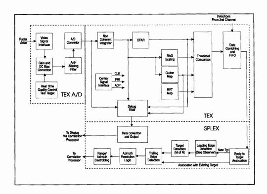
FIGURE 2-2. RDX FUNCTIONAL BLOCK DIAGRAM
