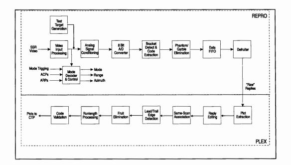
(5) **Thresholding.** The 8-bit data produced by the A/D converter is compared against a user selectable amplitude threshold and produces a 1-bit pulse train that is used in all subsequent processing. These pulses are then subjected to a width thresholding process where pulses shorter than a user selectable time are deleted and extremely long pulses are truncated.
