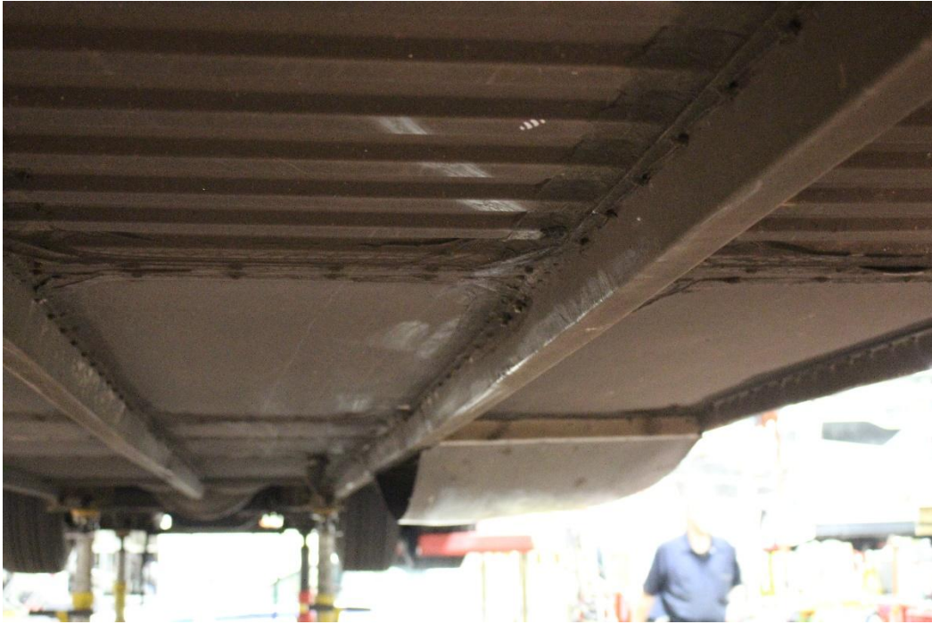
Photo #11: View of the undercarriage of the transit bus showing witness marks left by the pedestrian.
