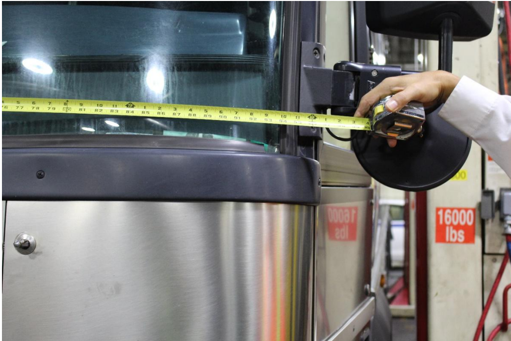
Photo #5: Measuring the overall width of the transit bus in the front. The transit bus is 8 ½ feet wide.
