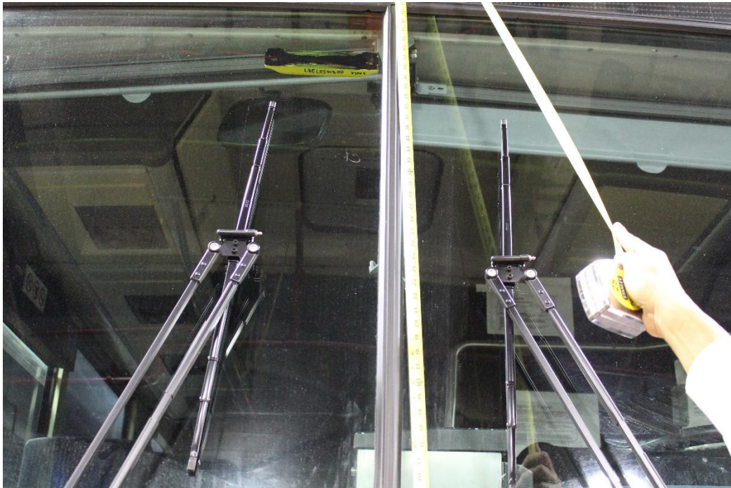
Photo #4: The front windshield's overall height was measured at 4 feet and 1 inch.
