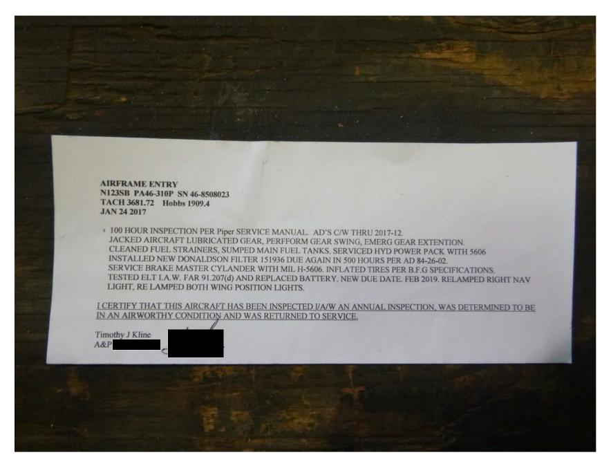
Photo 3 - Airframe 100 hour inspection
