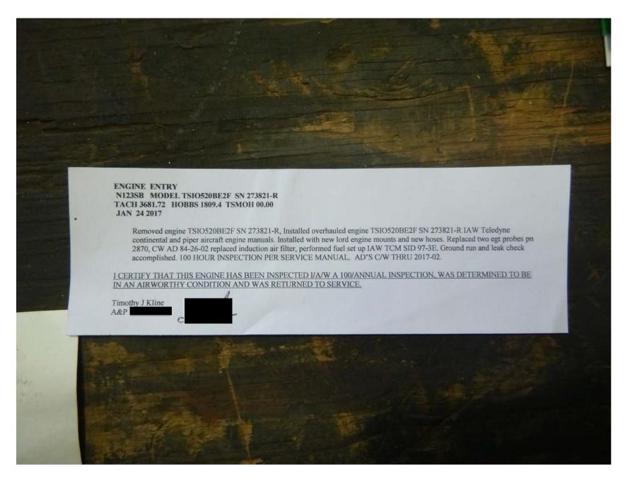
**Photo 2 - Engine 100 hour inspection**
