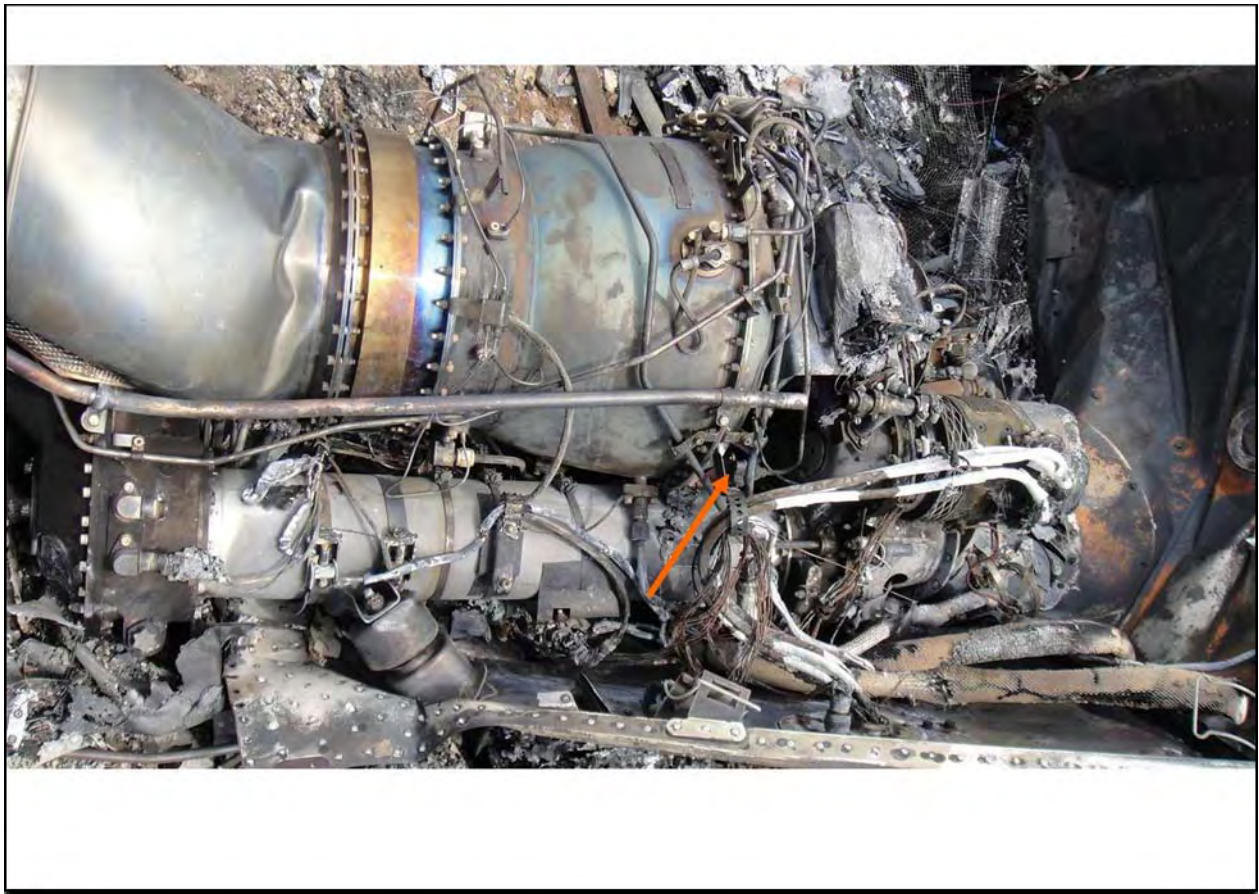
Photo 1. Engine at Accident Site (red arrow points to jet union)
