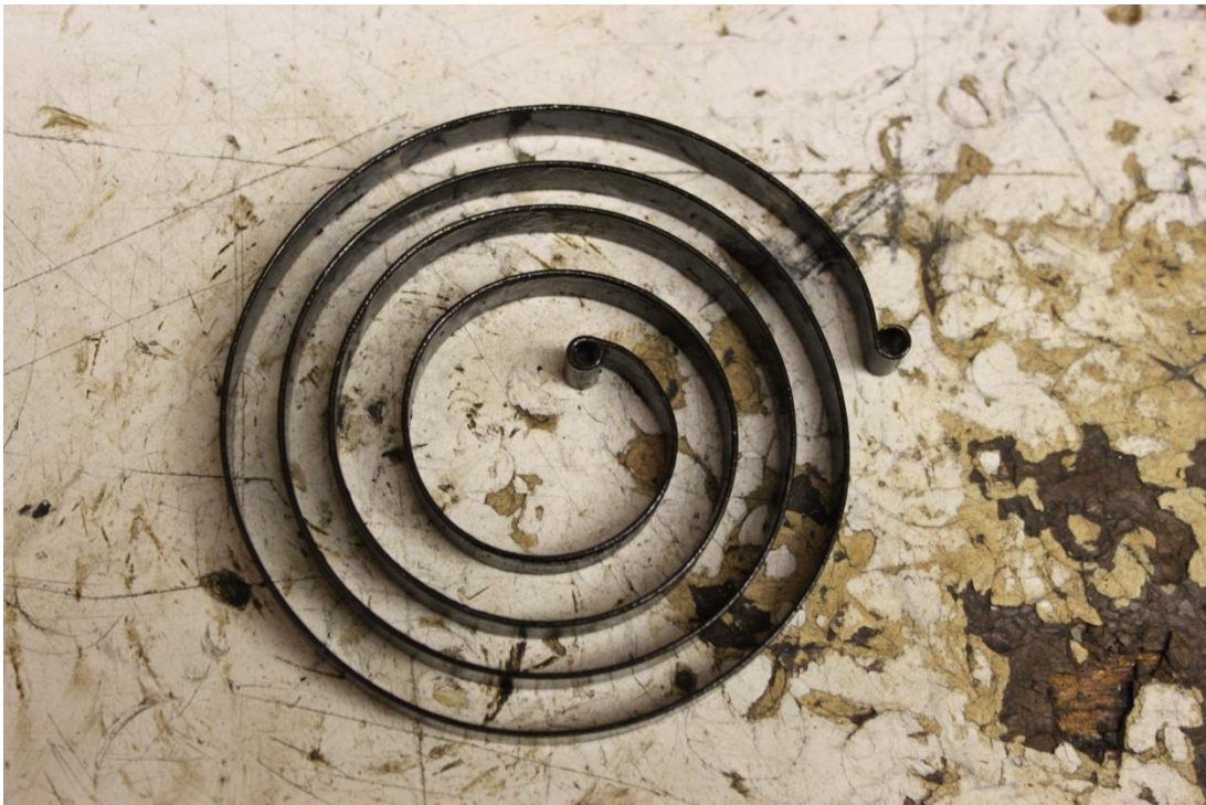
Figure 2: Left Magneto Impulse Coupling Spring
