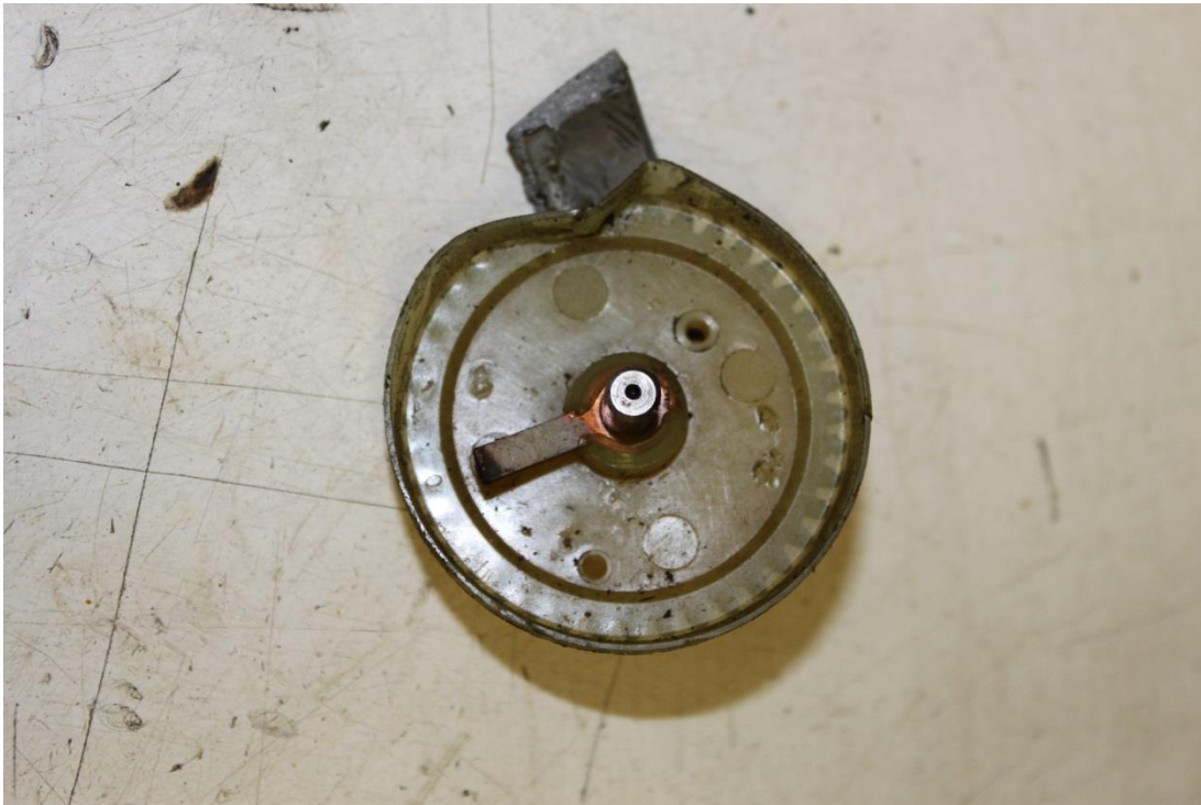
Figure 13: Right Magneto Distributor Gear and Electrode
