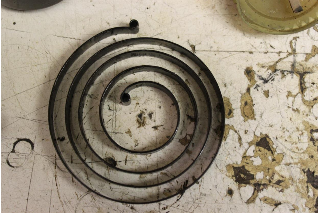
Figure 9: Right Magneto Impulse Coupling Spring
