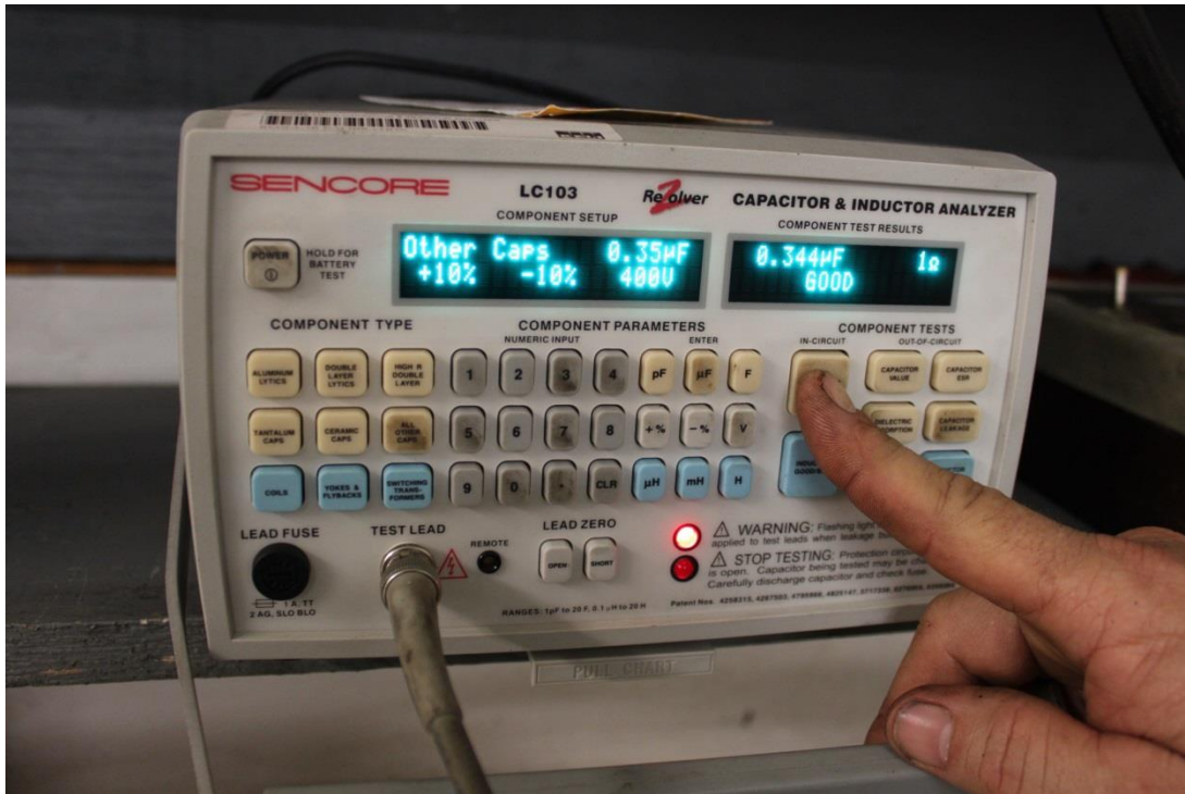
Figure 15: Test Results of Right Capacitor
