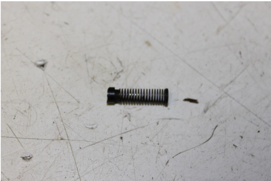
Figure 14: Right Magneto Carbon Brush and Spring
