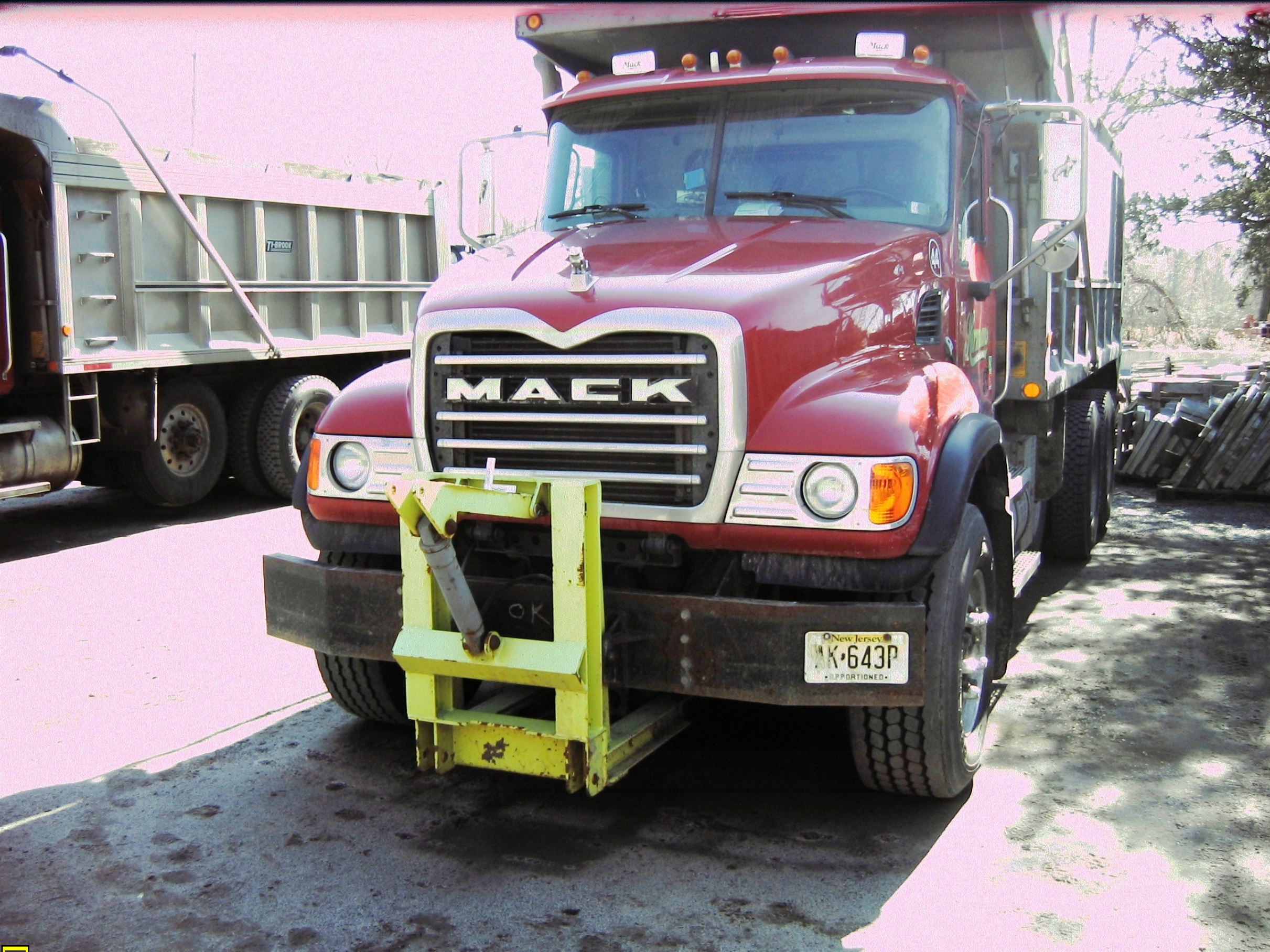
Photograph #1 - Snow Plow Device on Front of Truck
