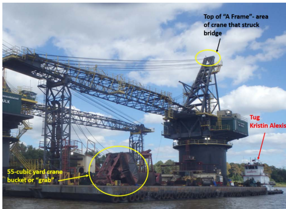
Figure 3. Photo of crane barge Mr Ervin faced up to the Kristin Alexis . (Source: Coast Guard)
