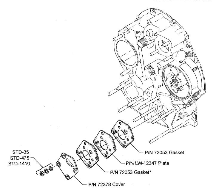
\* Replaced by gasket specified by airframe or propeller governor manufacturer when propeller governor installed.
