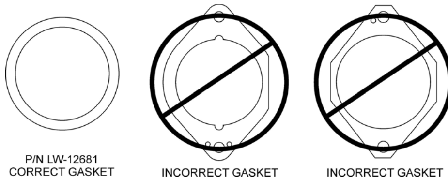
Figure 1 Correct and Incorrect Gaskets
