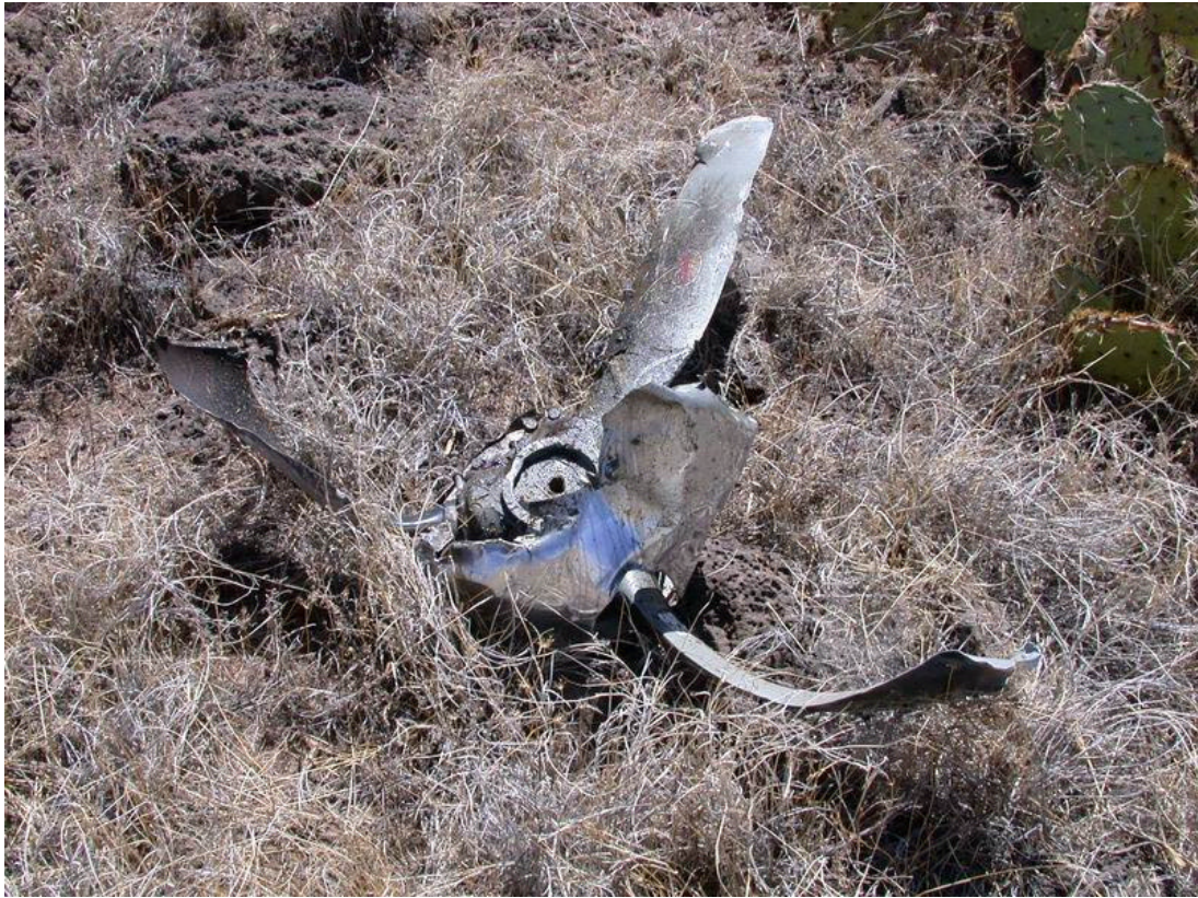
General view of propeller and blade damage.
