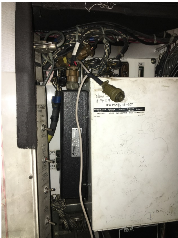
Figure 2. Downloading Amtrak 145's locomotive event recorder.
