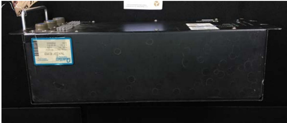
Figure 1. Photo of locomotive 4214's Quantum event recorder.
