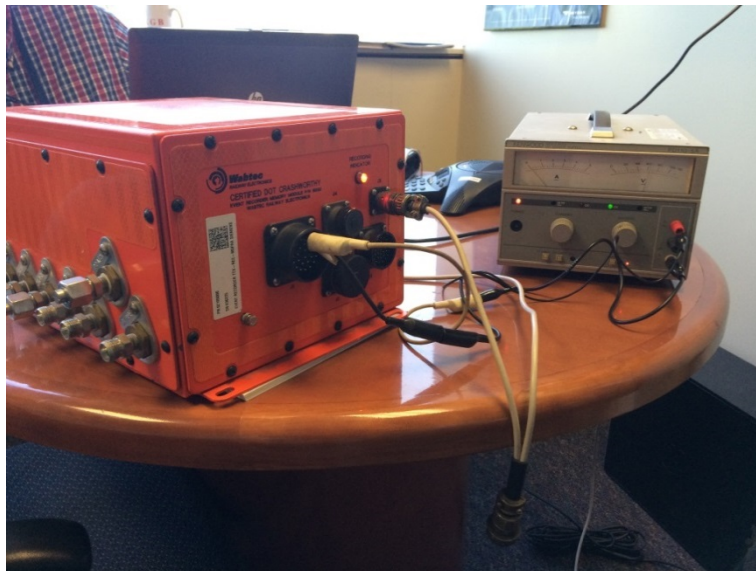
Figure 1. Downloading Amtrak 601's locomotive event recorder.
