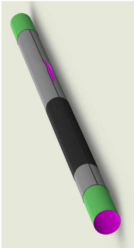
(above) ruptured segment out of trench. Polyethylene tape wrap coating (black) is only partially shown but covered the entire pipeline.
