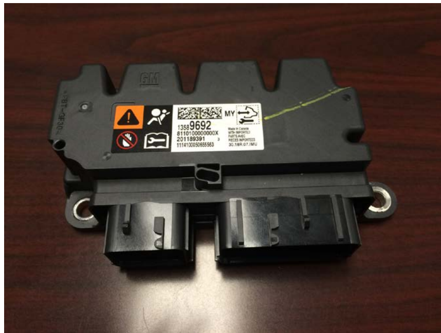
Figure 2: ACM extracted from 2014 Cadillac CTS.
