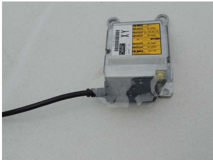
Figure 3: 2010 Toyota Prius ACM during bench-top download.
