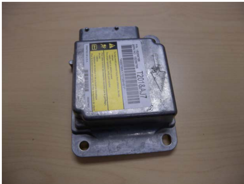
Figure 1: ACM extracted from 2007 Chevy Uplander.
