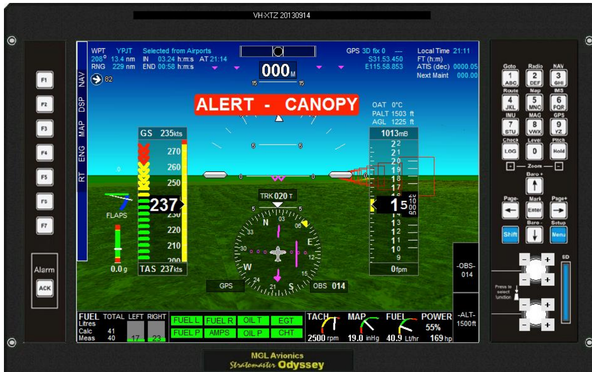
Example EFIS Warning in John Smith's and Gary Weeks' Lancair Legacys (VH-XTZ and VH-ZYA)
