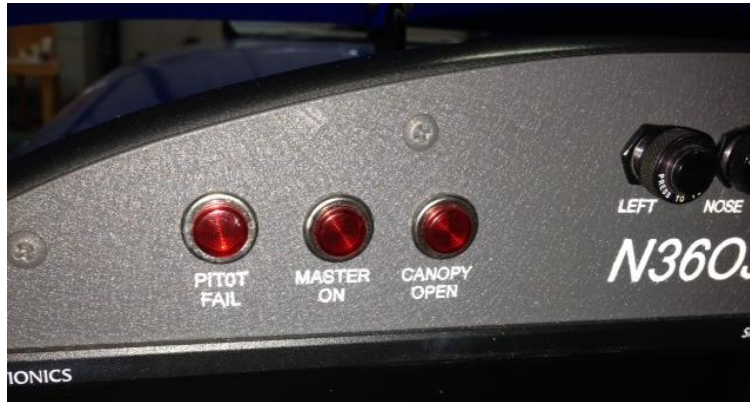
Example Canopy Unsafe Warning Light in Jack Addison's Lancair 360
