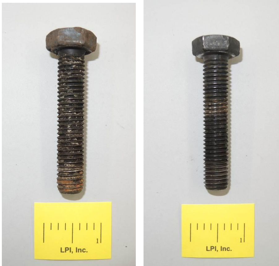
Fig. 2 Bolt 3(left) and bolt 4 (right) as-received.
