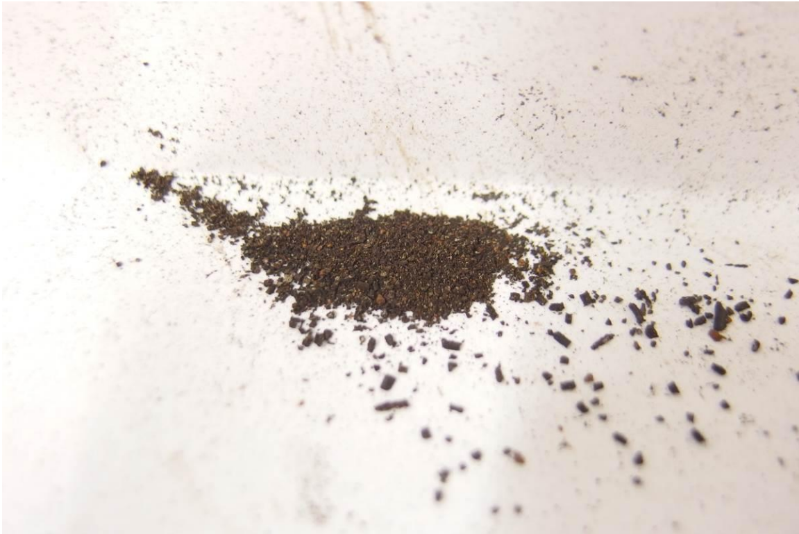
Fig. 5 Debris collected from the thread shank of bolt 3.
