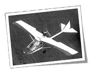
We took our Mark III Classic, added the aerodynamic expertise BarnabyWainfan, threw in a dash of ergonomics and cout with the Mark III Xtra while retaining the excellent STOL performance of the Classic. The Mark III Xtra, along wi Kolb aircraft, has folding wings and tails which allows for easy set-up and take-down. The tail folds up and the wings back. The process can be done in about 15 minutes. No tools or brackets are required. Everything stores right or airframe.
