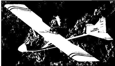
The FireStar II is designed to carry two people and give great climb performance with the very popular Rotax 503 engine. The FireStar II was designed specifically to use the Rotax 503 since this engine has proven to be the most reliable two stroke engine that Rotax makes.
