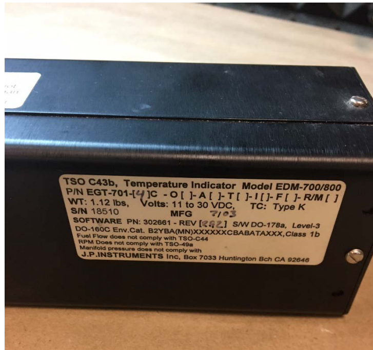
Figure 2. View of side of engine data monitor
