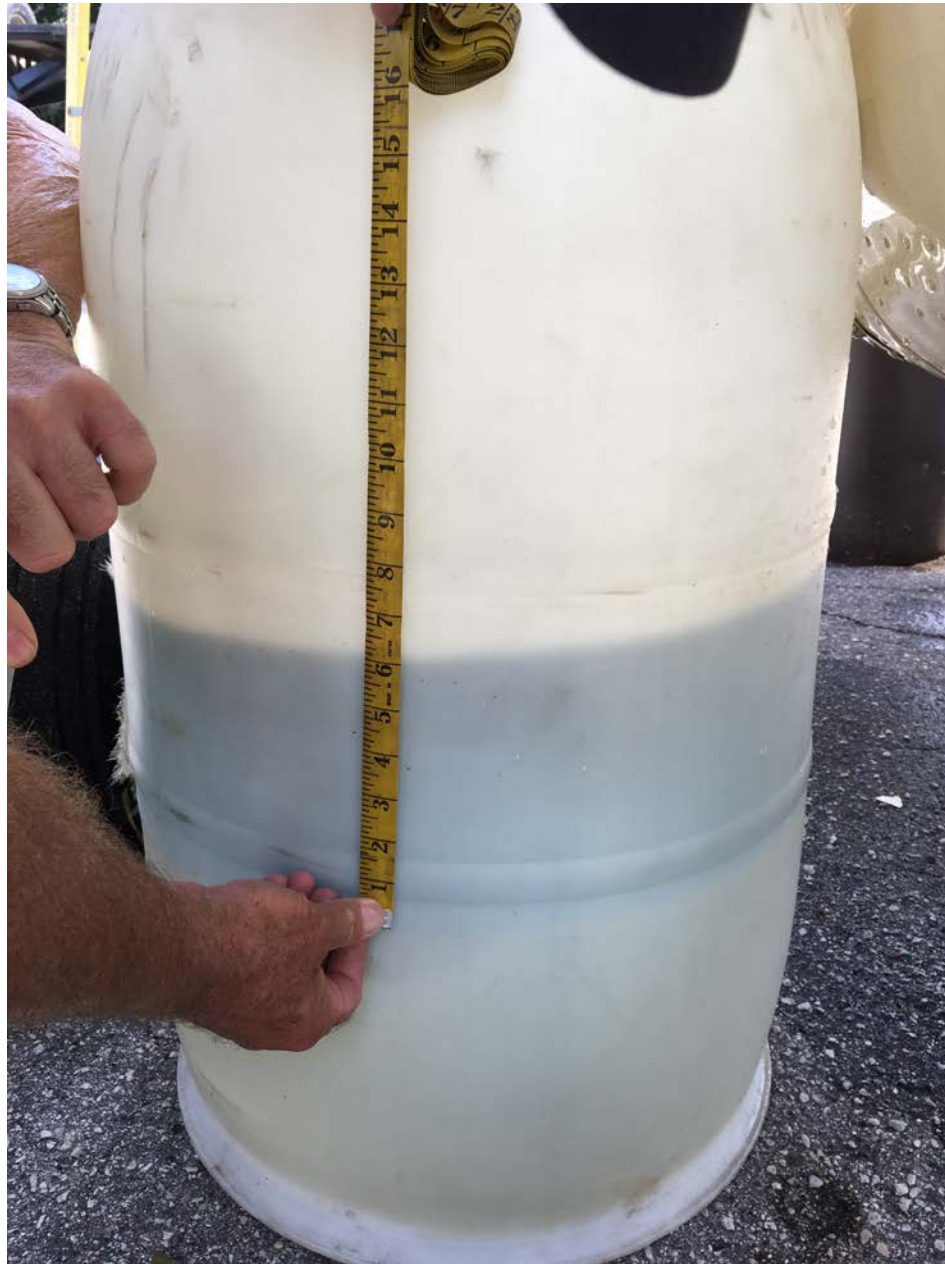
Photo 2 – Fuel and Water removed from fuel tanks
